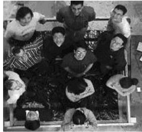
Figure C3.1-1—Live Load of 50 psf
