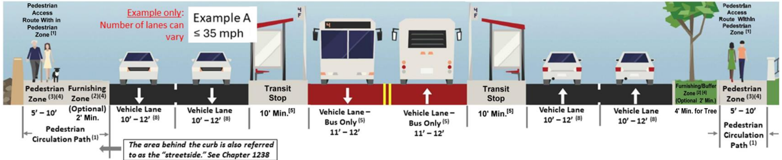
Exhibit 1231-6 Cross Sections Featuring Transit Facilities
