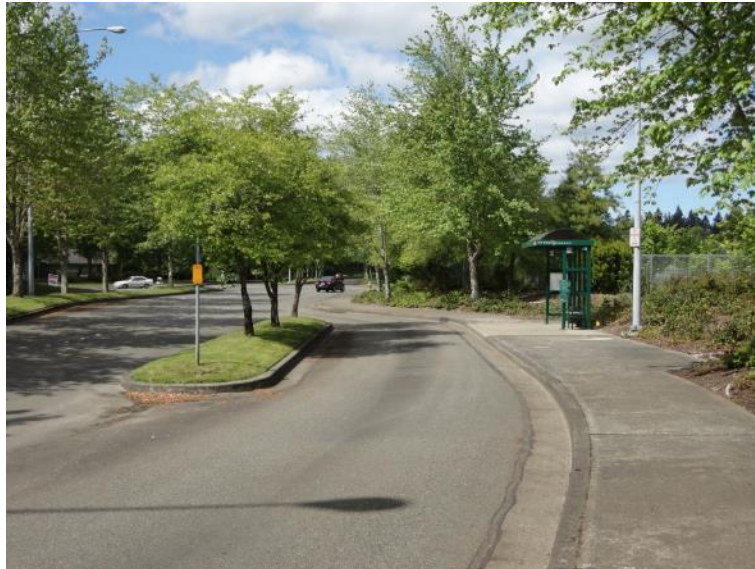
Bus Pullout with Longitudinal Island
