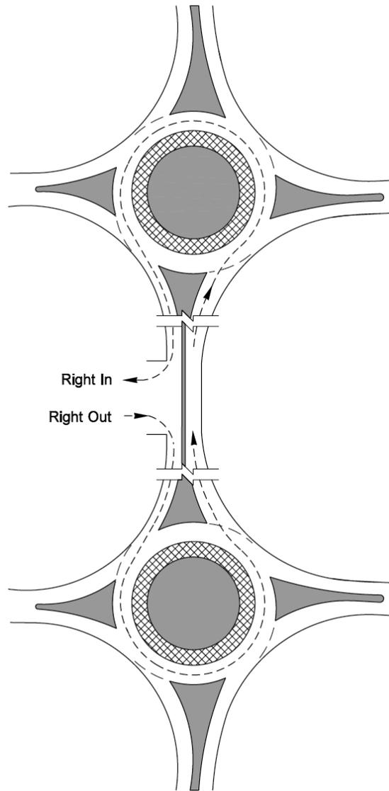
Left-turn access between roundabouts using U-turns at the roundabouts.
