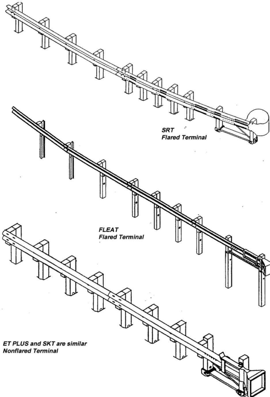
**Beam Guardrail Terminals**
