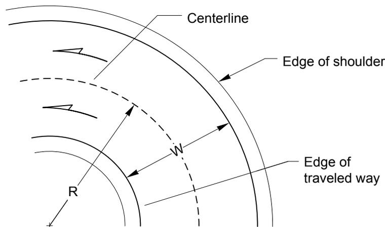
**Traveled Way Width for Two-Lane One-Way Turning Roadways**
