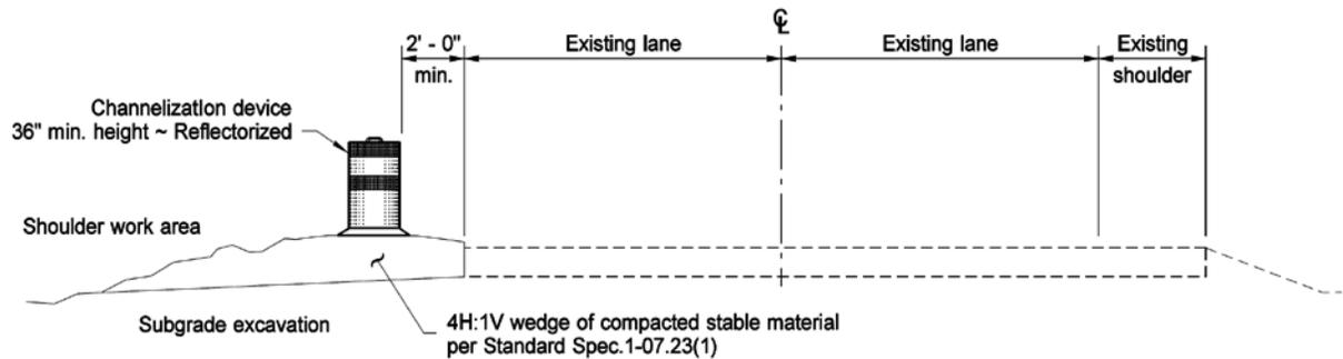
**Abrupt Edge Pavement Drop-Off Protection**
