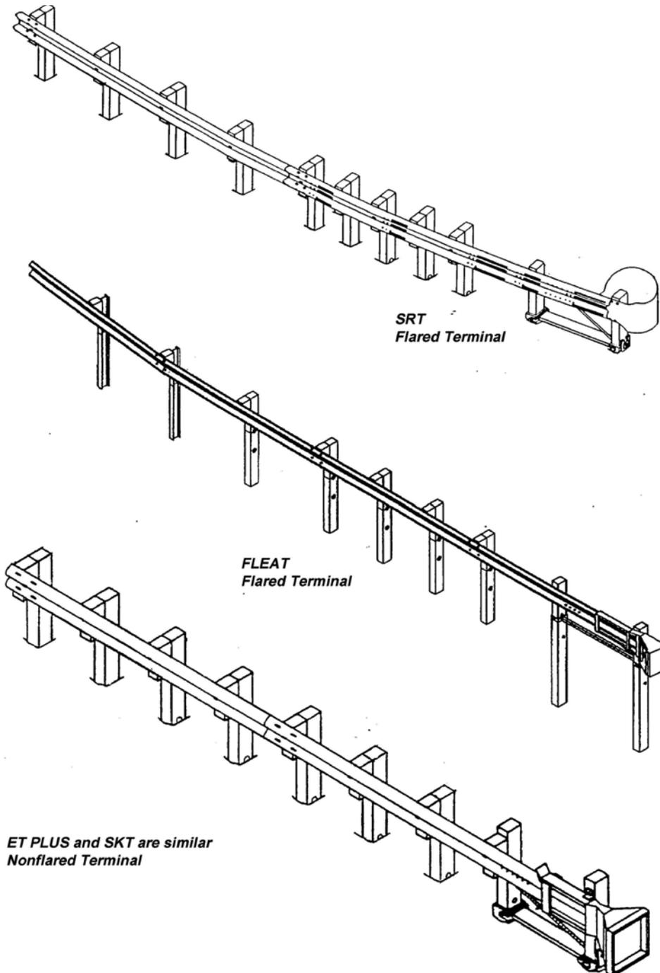
**Beam Guardrail Terminals**
