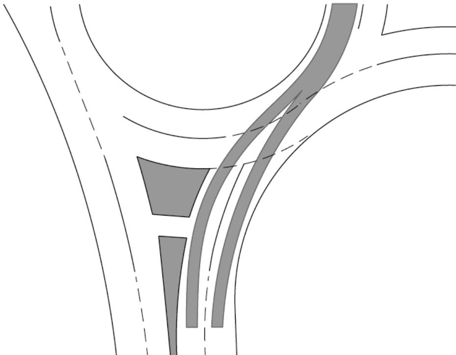
**Entry Design With Path Overlap (Undesirable)**
