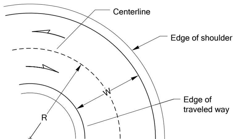
**Traveled Way Width for Two-Lane Two-Way Turning Roadways**
