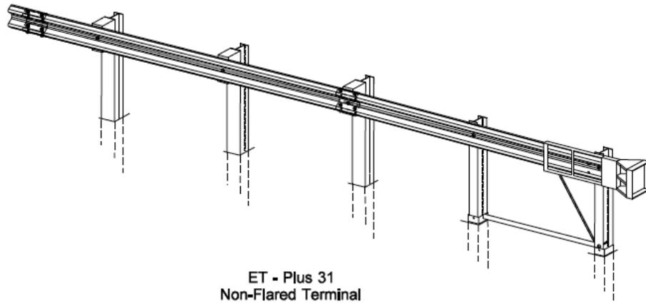
**Beam Guardrail Terminals**
