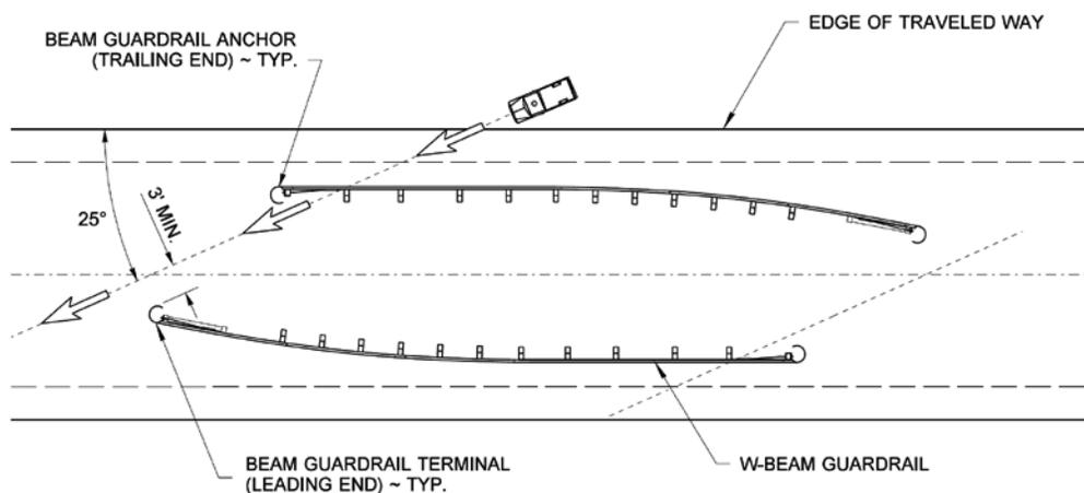
**W-Beam Guardrail Trailing End Placement for Divided Highways**
