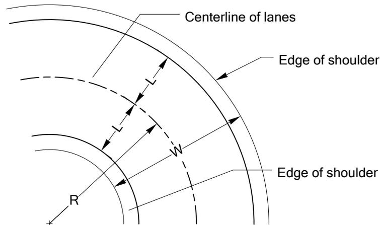
**Minimum Total Roadway Widths for Two-Lane Two-Way Highway Curves:
