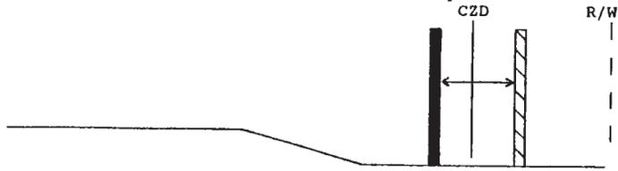
III. Situations in which the Control Zone Distance extends beyond the R/W. Relocating the utility object outside the R/W is required for CZ compliance. The utility object can be relocated to the R/W line.
