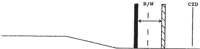
IV. Situations in which the Control Zone Distance is located within the R/W. The terrain or other physical features prevent relocation outside the Control Zone.
