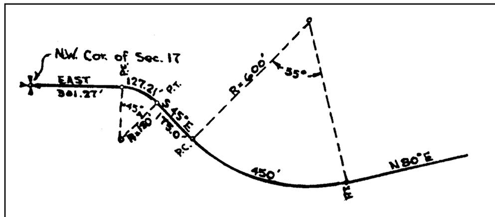
A compound curve is one in which the radius of the curve is changed somewhere along the arc without the intervention of a tangent course.
