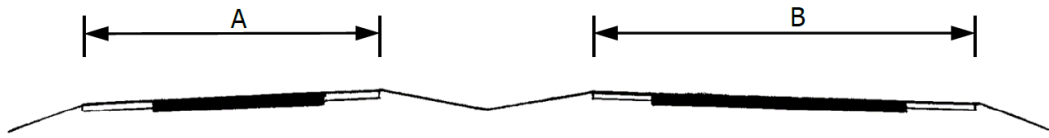
Figure 64. Cross-section view of two approach roadways that are carried across one bridge.
