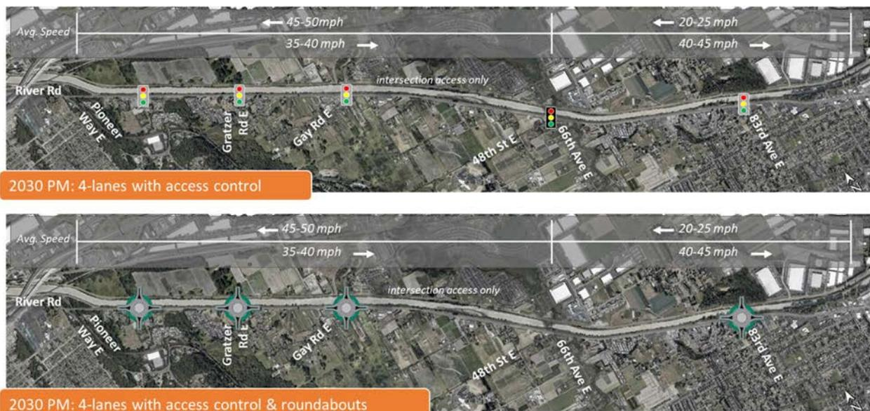
Figure 8 – Operations for 4-lane option with signalized and roundabout access control
