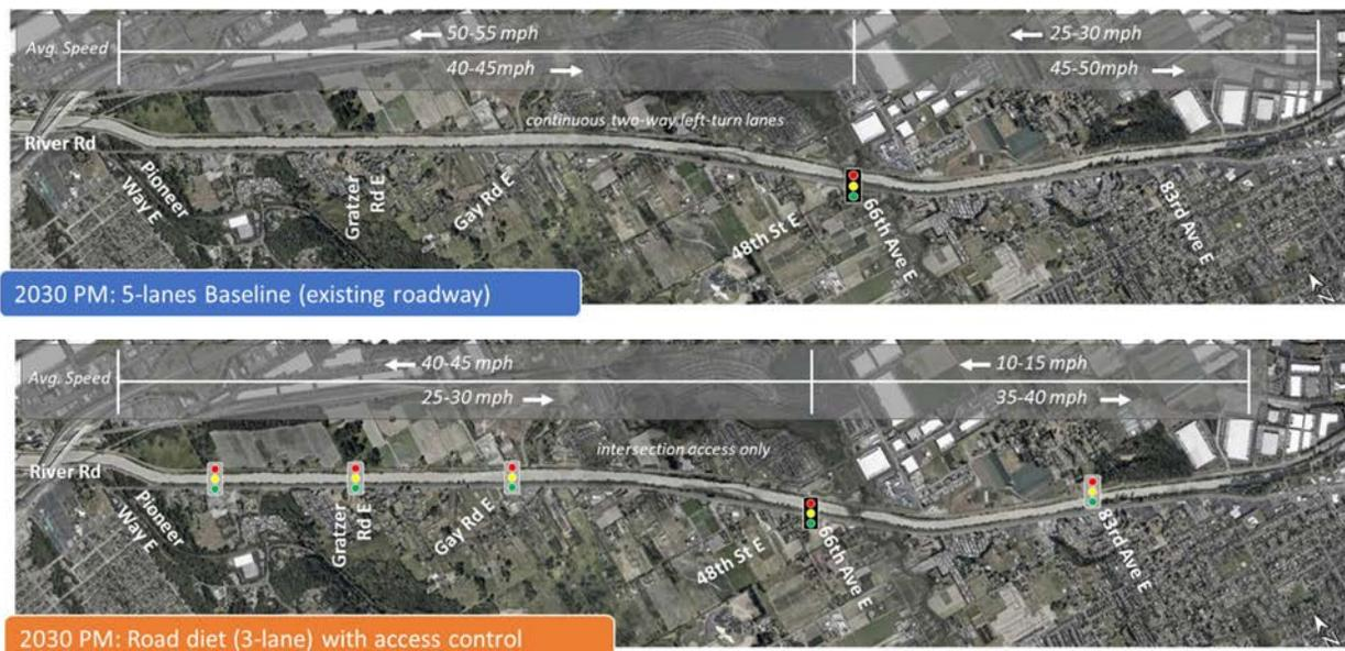
Figure 7 – Operations for existing roadway and three-lane option
