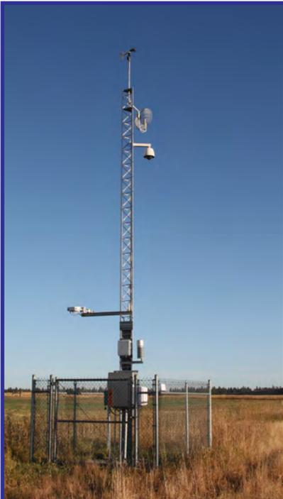
*WSDOT has invested in advanced technologies designed to monitor, report and forecast road related weather conditions through the use of Road Weather Information Systems (RWIS).*
