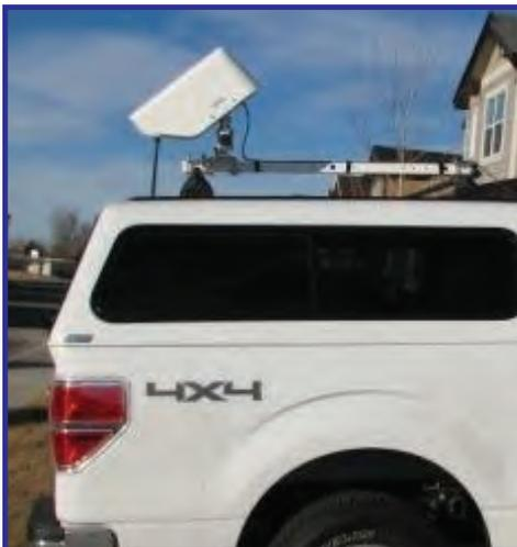
*Example of a mobile weather system equipped on a vehicle.*
