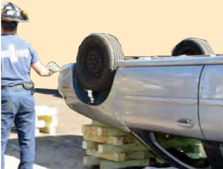
*Cribbing is an essential tool used during vehicle rescue operations to redistribute the weight of objects and provide temporary support*
