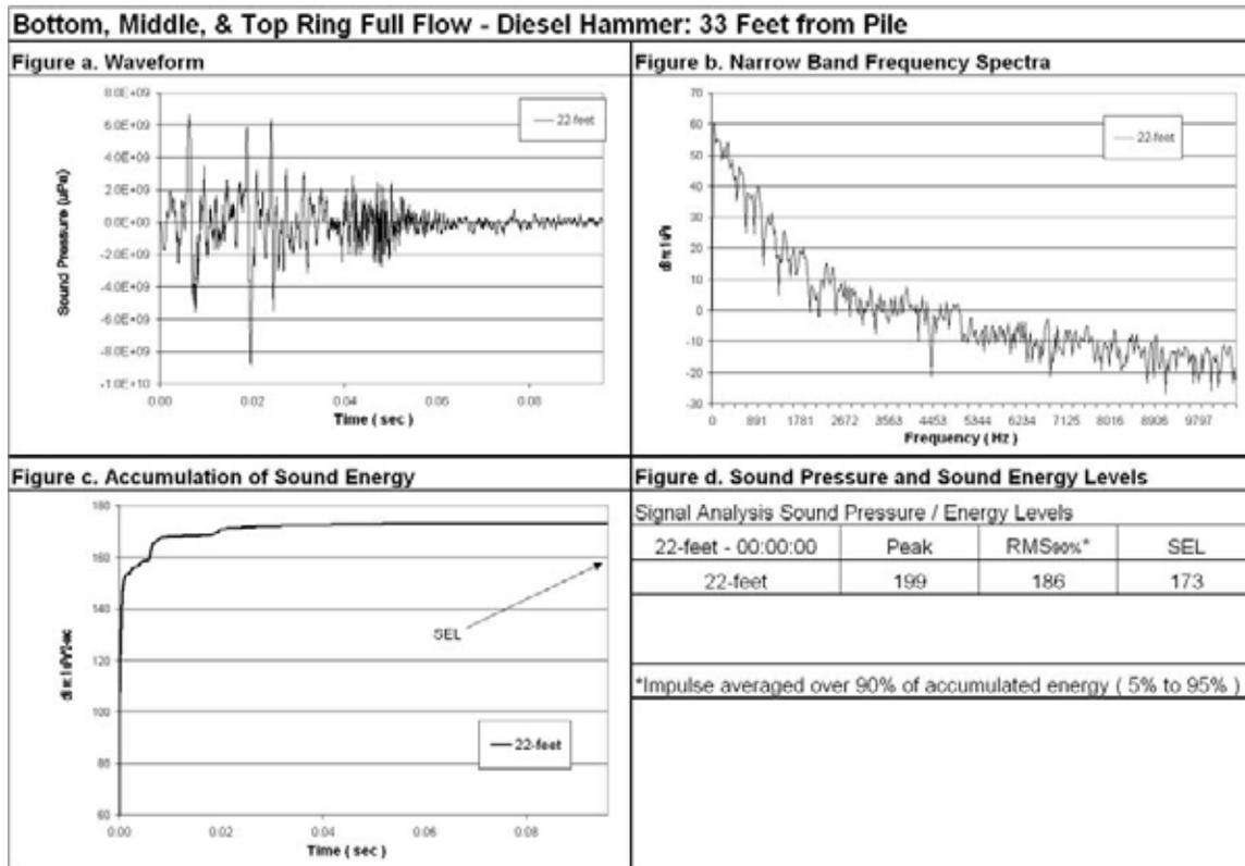
**Figure 64 Waveform Analysis for Pile Number 1, 22-feet Deep, 33-Feet from Pile, Bottom Ring, Middle, and Top Ring Full Flow**
