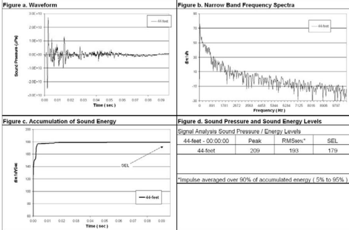
**Figure 75 Waveform Analysis for Pile Number 2, 44-Foot Deep (Bottom), 33-Feet from Pile, All Rings Off (Final).**
