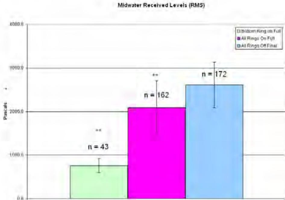
**Figure 41. Pile 8, midwater average RMS received levels. Error bars represent one standard deviation. \* = Significant compared to bubbles off initial (p<0.05). \*\* Significant compared to bubbles off final (p<0.05)**
