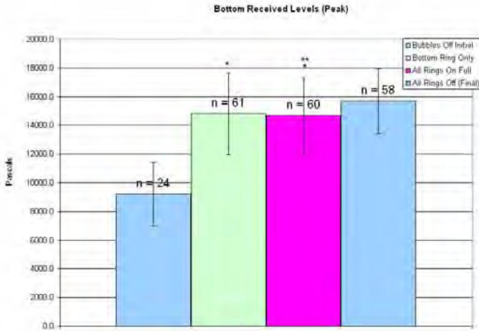
**Figure 18: Pile 3, bottom average peak received levels. Error bars represent one standard deviation. \* = Significant compared to bubbles off initial (p<0.05). \*\* Significant compared to bubbles off final (p<0.05)**
