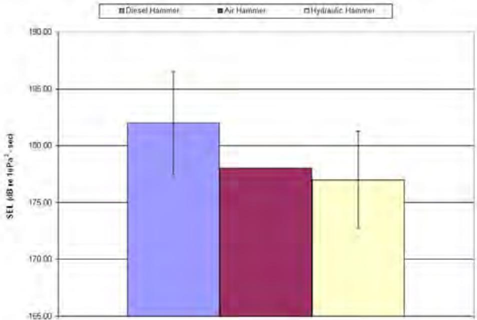
**Figure 48. SEL midwater received values for each hammer type, all bubble rings off. Error bars are  $\pm$  one standard deviation. SEL for the air hammer represents only one sample.**
