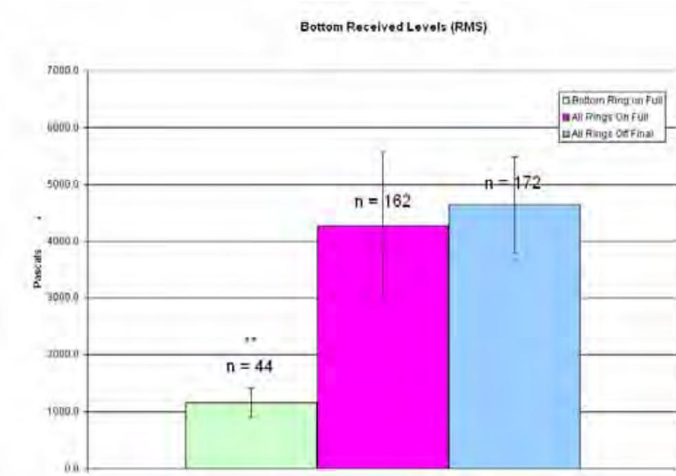
**Figure 33. Pile 6, bottom average RMS received levels. Error bars represent one standard deviation. \* = Significant compared to bubbles off initial ( $p < 0.05$ ). \*\* Significant compared to bubbles off final ( $p < 0.05$ )**
