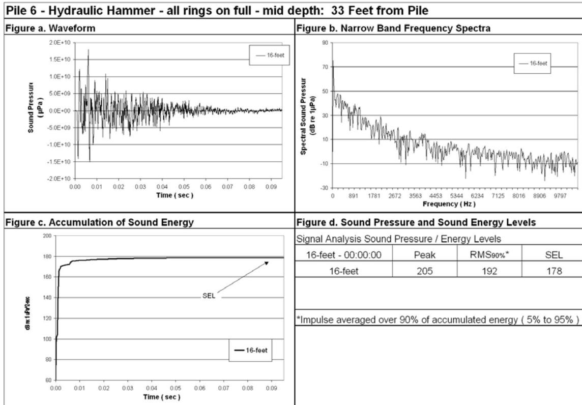
**Figure 98: Waveform Analysis for Pile Number 6, 16-Foot Deep, 33-Foot from Pile, All Rings On Full.**
