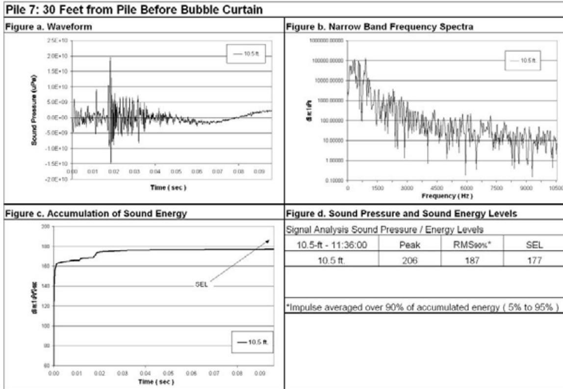
**Figure 50: Results of Sound Pressure Levels without Bubble Curtain**
