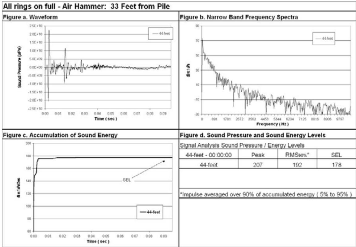
**Figure 73 Waveform Analysis for Pile Number 2, 44-Foot Deep (Bottom), 33-Foot from Pile, All Rings On Full.**
