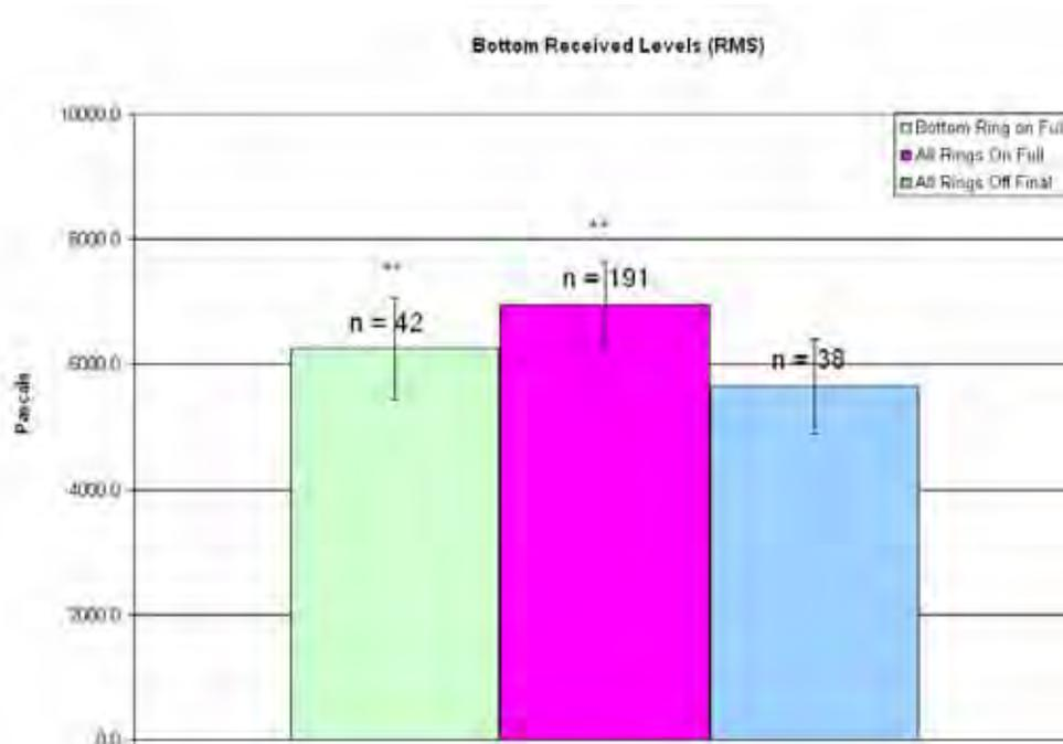
**Figure 29. Pile 5, bottom average RMS received levels. Error bars represent one standard deviation. \* = Significant compared to bubbles off initial ( $p < 0.05$ ). \*\* Significant compared to bubbles off final ( $p < 0.05$ )**
