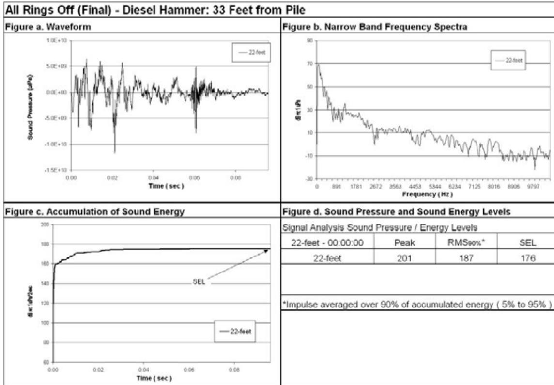
**Figure 66 Waveform Analysis for Pile Number 1, 22-feet Deep, 33-Feet from Pile, All Rings Off (Final).**
