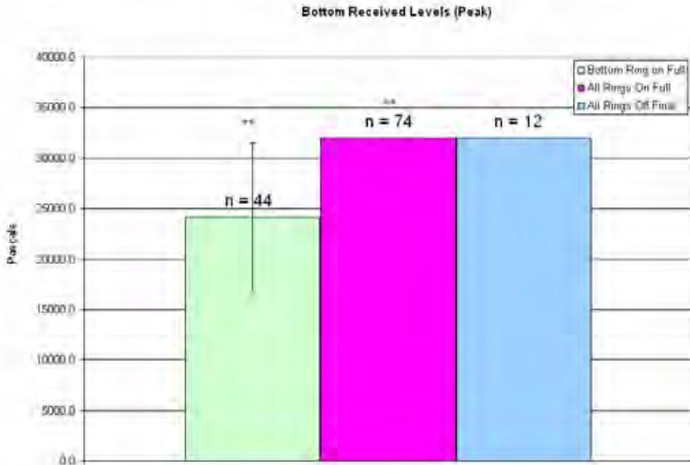
**Figure 23: Pile 4, bottom average peak received levels. Error bars represent one standard deviation. \* = Significant compared to bubbles off initial (p<0.05). \*\* Significant compared to bubbles off final (p<0.05)**
