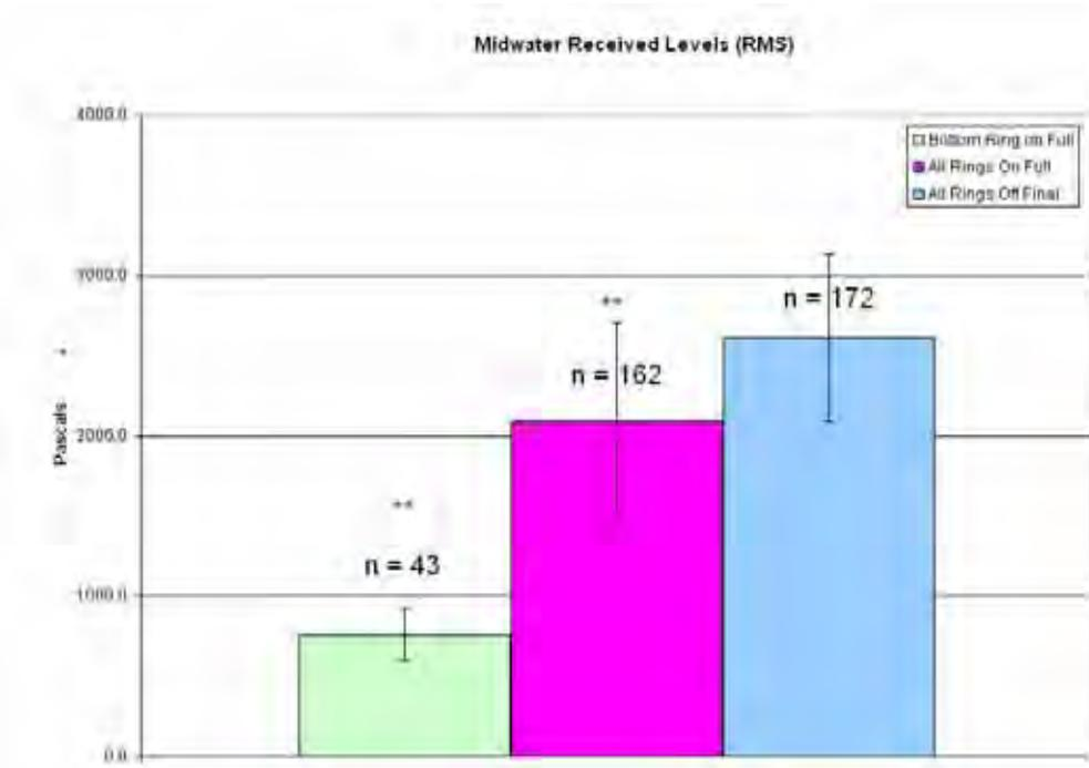
**Figure 32. Pile 6, midwater average RMS received levels. Error bars represent one standard deviation. \* = Significant compared to bubbles off initial ( $p < 0.05$ ). \*\* Significant compared to bubbles off final ( $p < 0.05$ )**
