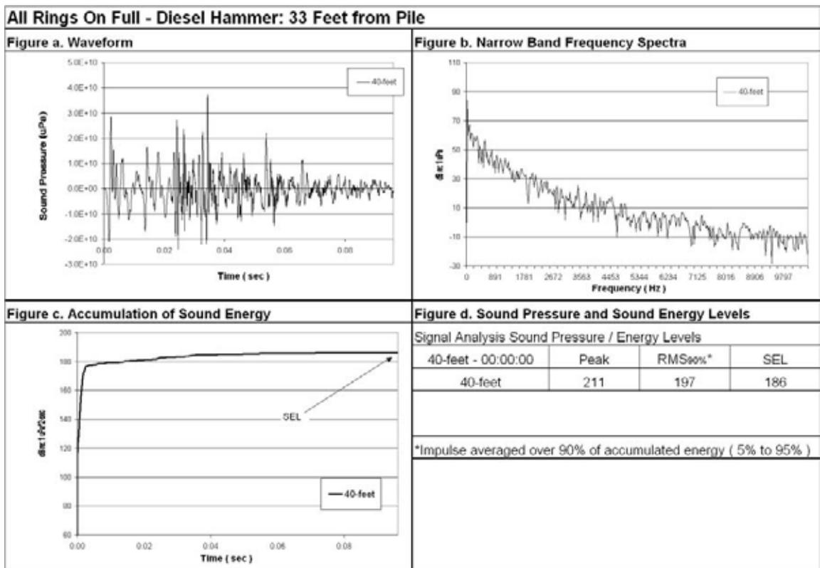
**Figure 105: Waveform Analysis for Pile Number 7, 40-Foot Deep (Bottom), 33-Foot from Pile, All Rings On Full.**
