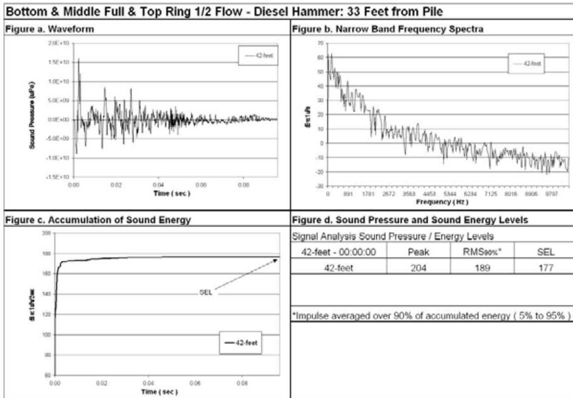
Figure 62 Waveform Analysis for Pile Number 1, 42-foot Deep (bottom), 33-Feet from Pile, Bottom Ring and Middle Full, Top Ring 1/2 Flow.
