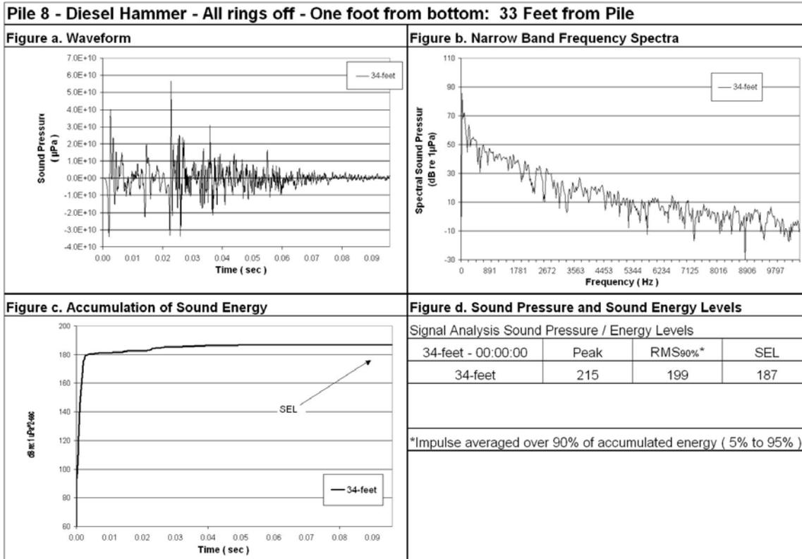
**Figure 111: Waveform Analysis for Pile Number 8, 34-Foot Deep (Bottom), 33-Foot from Pile, All Rings Off.**
