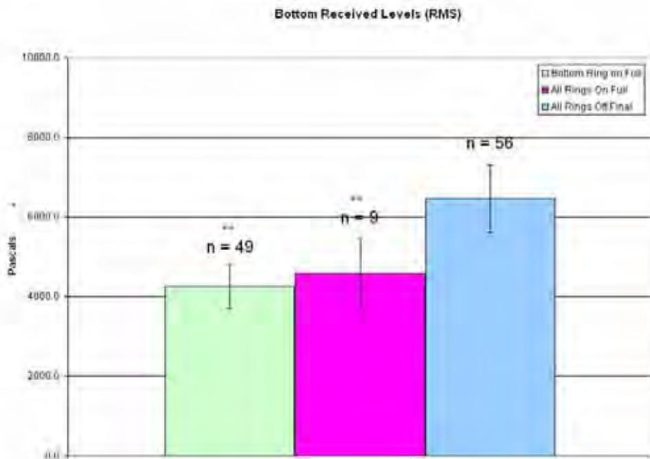
**Figure 42. Pile 8, midwater average RMS received levels. Error bars represent one standard deviation. \* = Significant compared to bubbles off initial (p<0.05). \*\* Significant compared to bubbles off final (p<0.05)**
