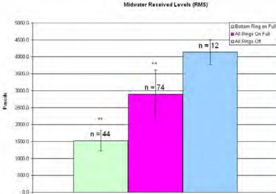
**Figure 24: Pile 4, midwater average RMS received levels. Error bars represent one standard deviation. \* = Significant compared to bubbles off initial ( $p < 0.05$ ). \*\* Significant compared to bubbles off final ( $p < 0.05$ )**
