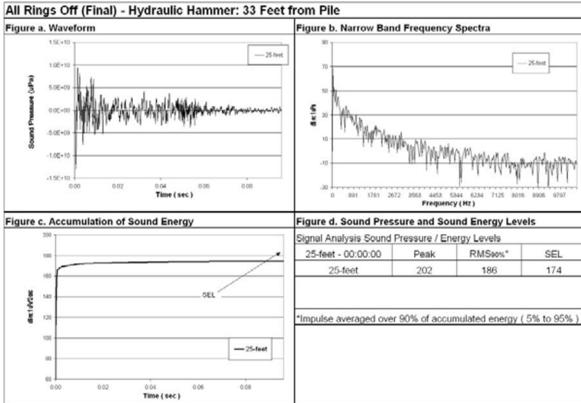
Figure 82 Waveform Analysis for Pile Number 3, 25-feet Deep, 33-Feet from Pile, All Rings Off (Final).
