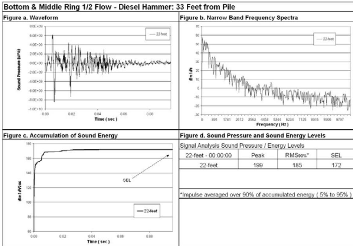
**Figure 56: Waveform Analysis for Pile Number 1, 22-feet Deep, 33-Feet from Pile, Bottom and Middle Ring 1/2 Flow.**
