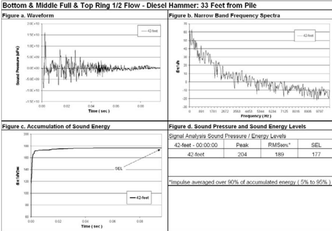
**Figure 63 Waveform Analysis for Pile Number 1, 42-feet Deep (bottom), 33-Feet from Pile, Bottom and Middle Ring Full, Top Ring 1/2 Flow**
