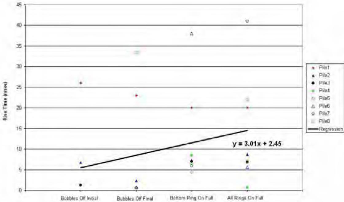
**Figure 44. Rise times for each bottom received level peak pile strike with linear regression line**
