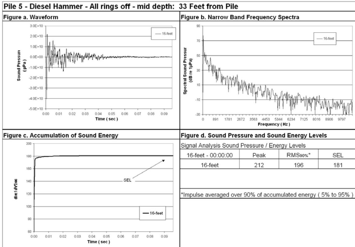
**Figure 94: Waveform Analysis for Pile Number 5, 16-Foot Deep (Bottom), 33-Foot from Pile, All Rings Off.**
