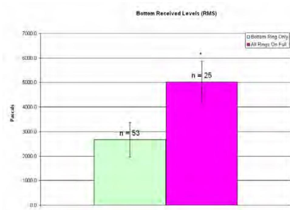
**Figure 38. Pile 7, bottom average RMS received levels. Error bars represent one standard deviation. \* = Significant compared to bottom ring on only ( $p < 0.05$ ).**
