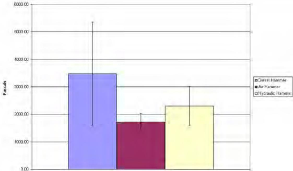
**Figure 47. Average RMS midwater received values for each hammer type, all bubble rings off. Error bars are  $\pm$  one standard deviation**
