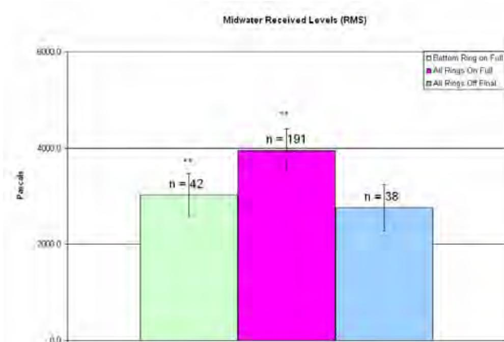
**Figure 28. Pile 5, midwater average RMS received levels. Error bars represent one standard deviation. \* = Significant compared to bubbles off initial ( $p < 0.05$ ). \*\* Significant compared to bubbles off final ( $p < 0.05$ )**
