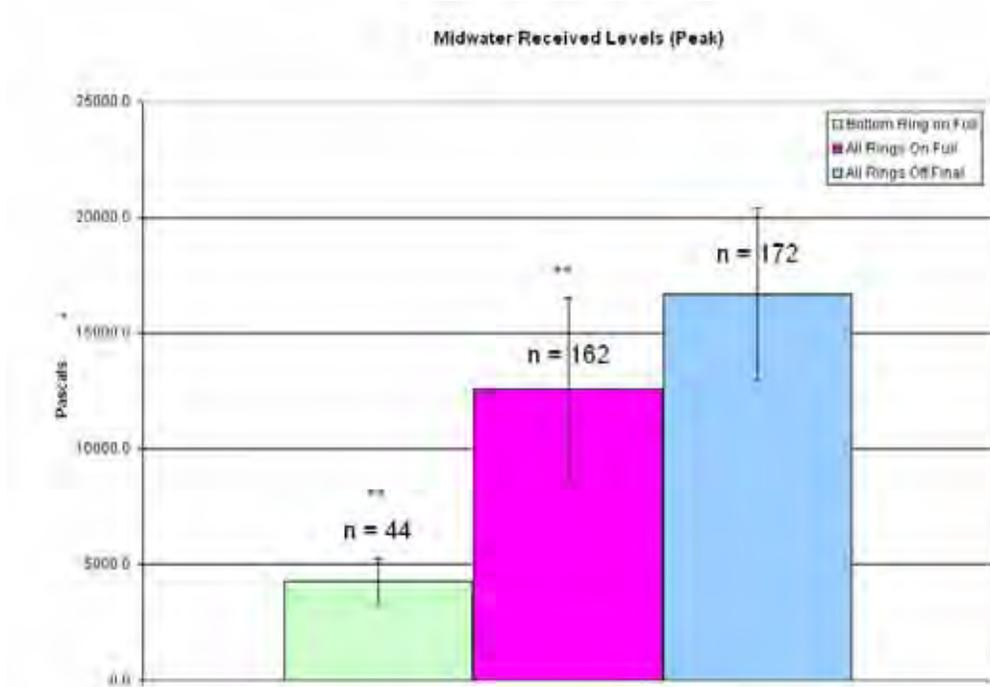
**Figure 30. Pile 6, midwater average peak received levels. Error bars represent one standard deviation. \* = Significant compared to bubbles off initial ( $p < 0.05$ ). \*\* Significant compared to bubbles off final ( $p < 0.05$ )**
