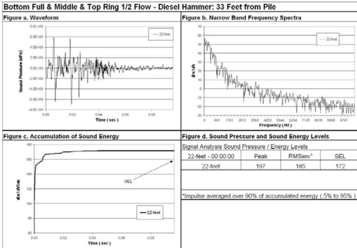
**Figure 60 Waveform Analysis for Pile Number 1, 22-feet Deep, 33-Feet from Pile, Bottom Ring Full Flow, Middle, and Top Ring 1/2 Flow.**
