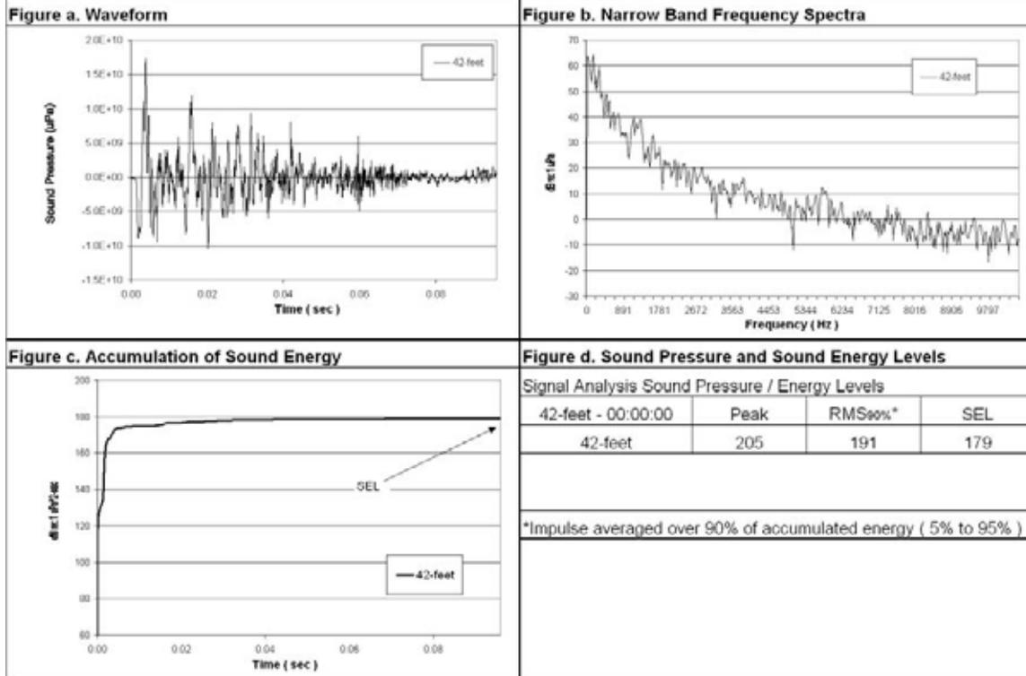
**Figure 53: Waveform Analysis for Pile Number 1, 42-feet (Bottom), 33-Feet from Pile, All Rings Off.**
