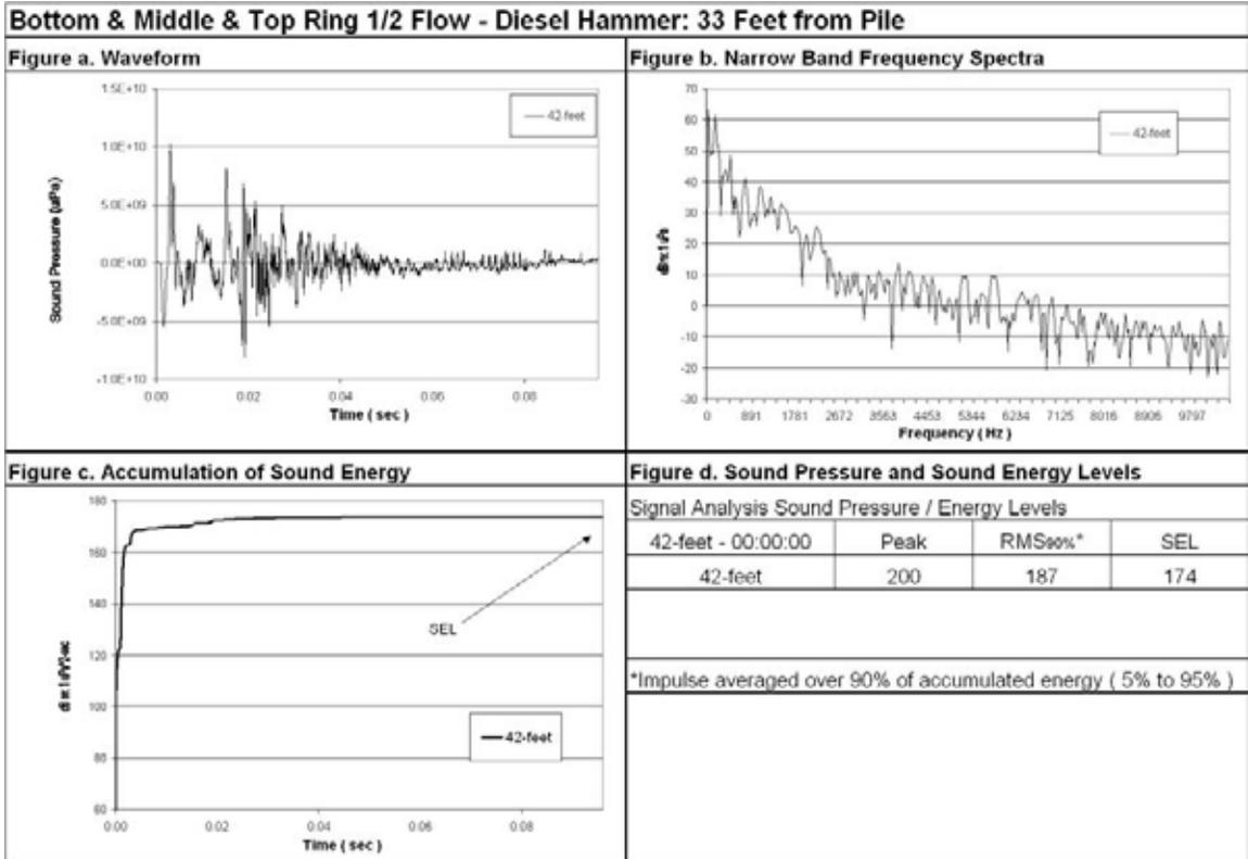
**Figure 59 Waveform Analysis for Pile Number 1, 42-foot Deep (bottom), 33-Feet from Pile, Bottom, Middle, and Top Ring 1/2 Flow.**
