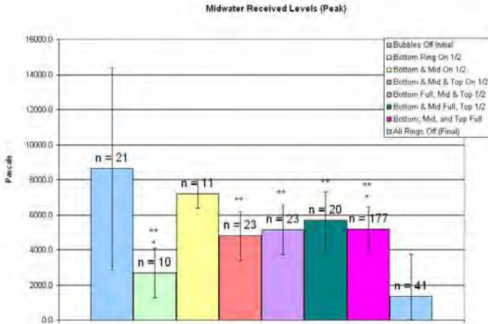
**Figure 7: Pile 1, midwater average peak received levels. Error bars represent one standard deviation. \* = Significant compared to bubbles off initial ( $p < 0.05$ ). \*\* Significant compared to bubbles off final ( $p < 0.05$ ).**
