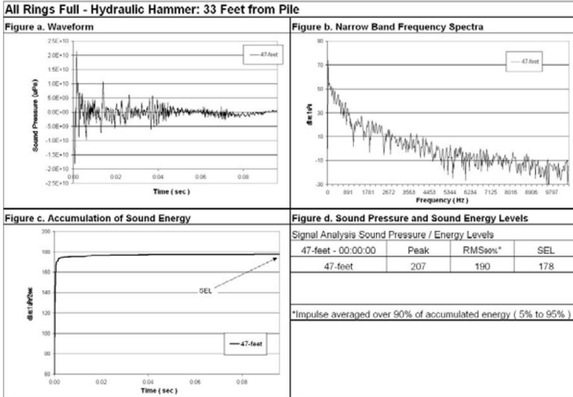
**Figure 81 Waveform Analysis for Pile Number 3, 47-foot Deep (Bottom), 33-Feet from Pile, All Rings Full.**
