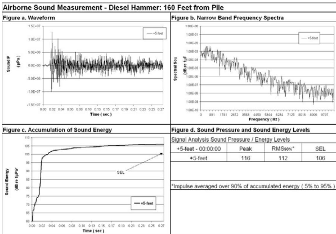
**Figure 49: Airborne Sound Levels of a Diesel Pile Driver and Steel Pile , 160 feet from pile.**
