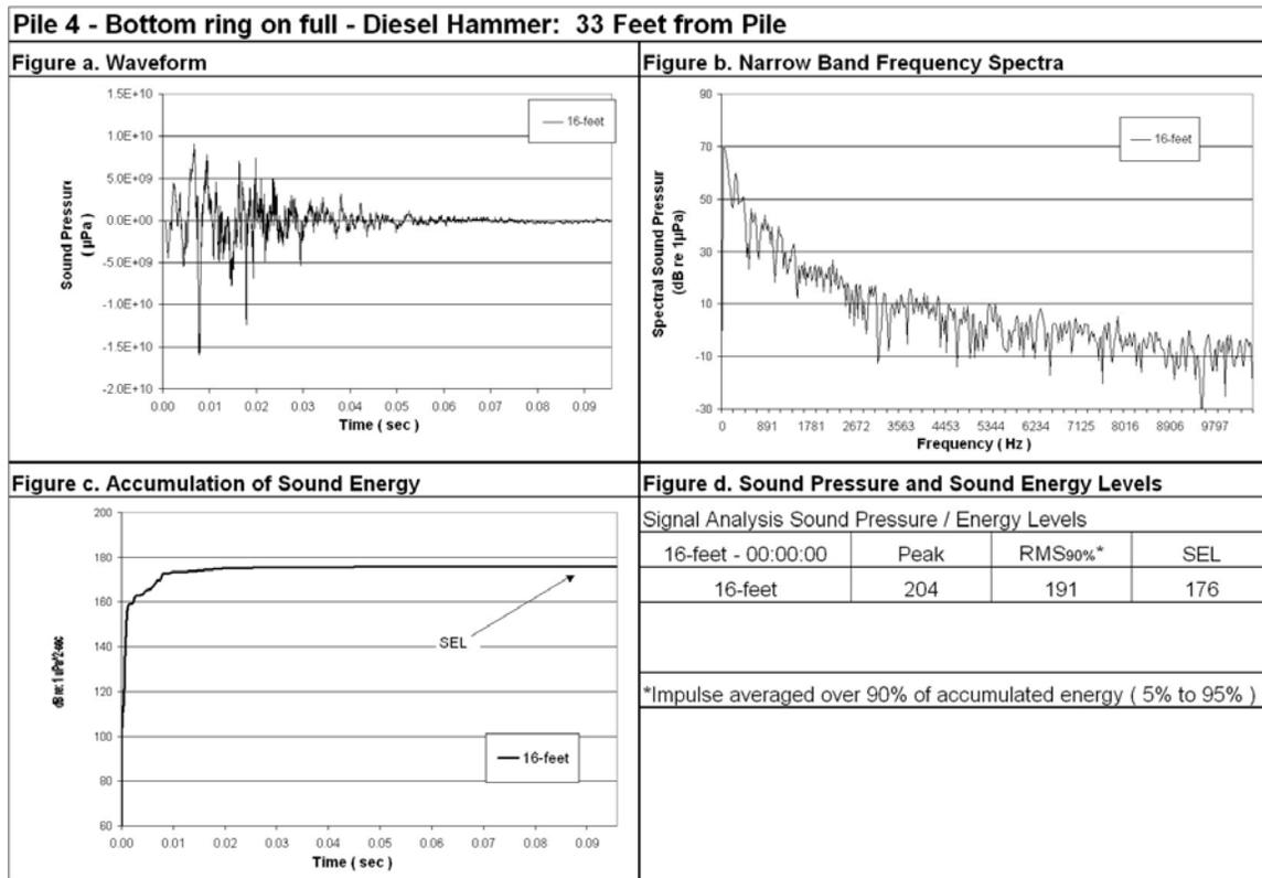
**Figure 84: Waveform Analysis for Pile Number 4, 16-Foot Deep, 33-Foot from Pile, Bottom Ring On Full.**
