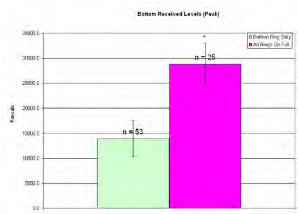
**Figure 36. Pile 7, bottom average peak received levels. Error bars represent one standard deviation. \* = Significant compared to bottom ring on only ( $p < 0.05$ ).**
