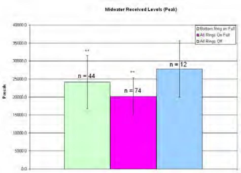
**Figure 22: Pile 4, midwater average peak received levels. Error bars represent one standard deviation. \* = Significant compared to bubbles off initial ( $p < 0.05$ ). \*\* Significant compared to bubbles off final ( $p < 0.05$ )**
