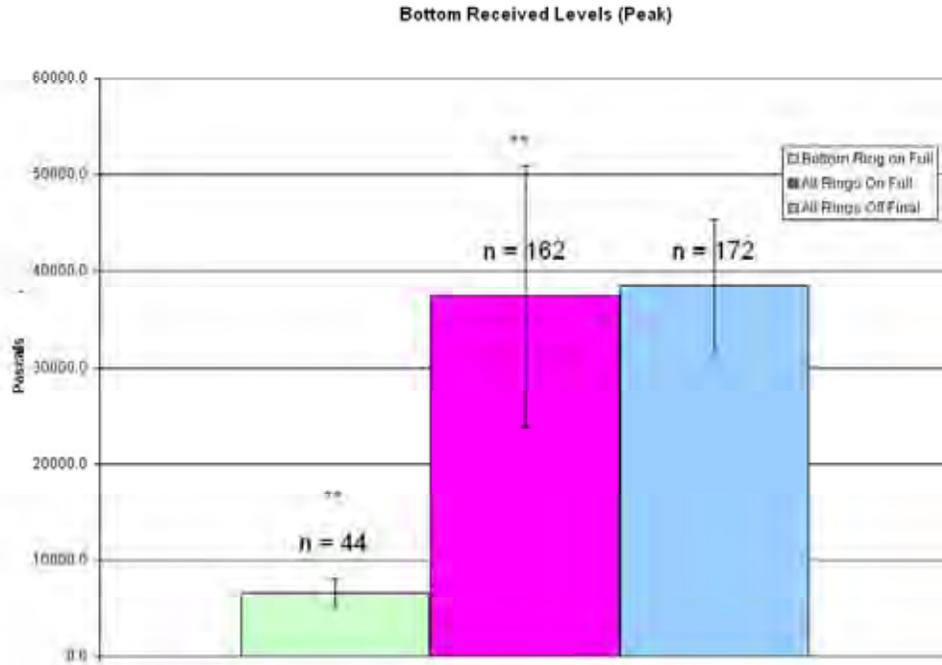
**Figure 31. Pile 6, bottom average peak received levels. Error bars represent one standard deviation. \* = Significant compared to bubbles off initial ( $p < 0.05$ ). \*\* Significant compared to bubbles off final ( $p < 0.05$ )**
