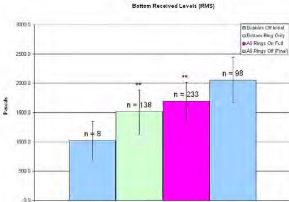
Figure 16: Pile 2, bottom average RMS received levels. Error bars represent one standard deviation. \* = Significant compared to bubbles off initial ( $p < 0.05$ ). \*\* Significant compared to bubbles off final ( $p < 0.05$ )
