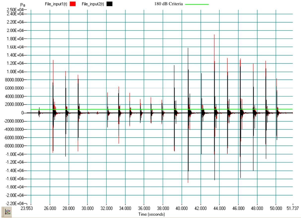
**Figure 5: Pile 1 Initial Pile Strikes with Bubble Curtain Off. (File\_input1(t) = bottom; File\_input2(t) = midwater)**
