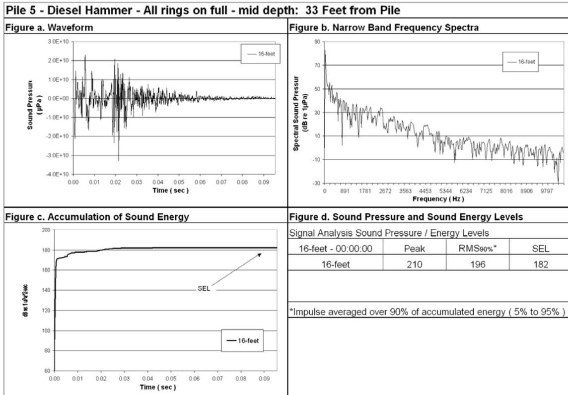
**Figure 92: Waveform Analysis for Pile Number 5, 16-Foot Deep, 33-Foot from Pile, All Rings On Full.**
