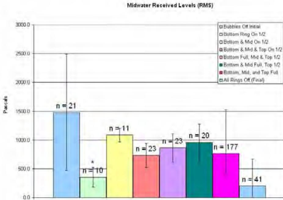
Figure 9: Pile 1, midwater average RMS received levels. Error bars represent one standard deviation. \* = Significant compared to bubbles off initial ( $p < 0.05$ ). \*\* Significant compared to bubbles off final ( $p < 0.05$ ).
