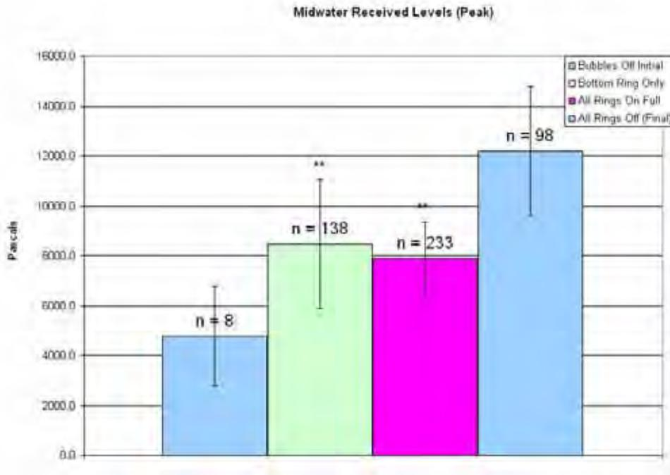
**Figure 13: Pile 2, midwater average peak received levels. Error bars represent one standard deviation. \* = Significant compared to bubbles off initial ( $p < 0.05$ ). \*\* Significant compared to bubbles off final ( $p < 0.05$ )**
