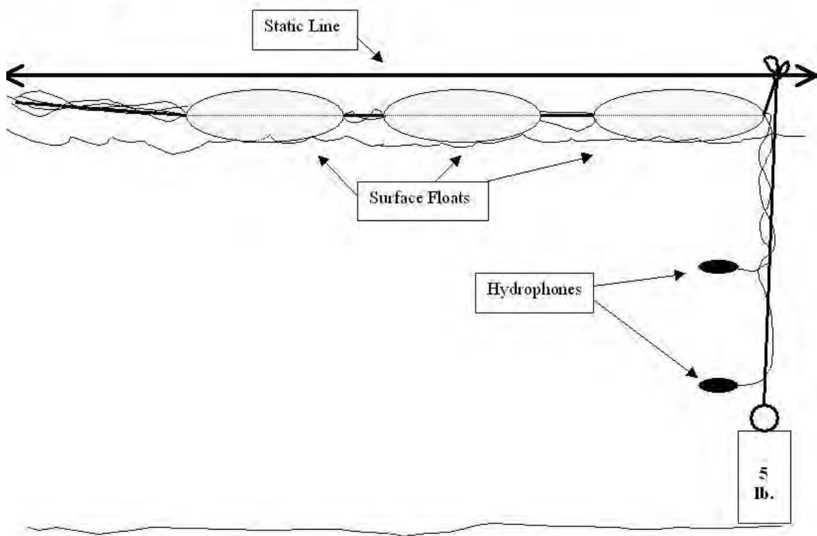
**Figure 3: Hydrophone Weight and Float System**
