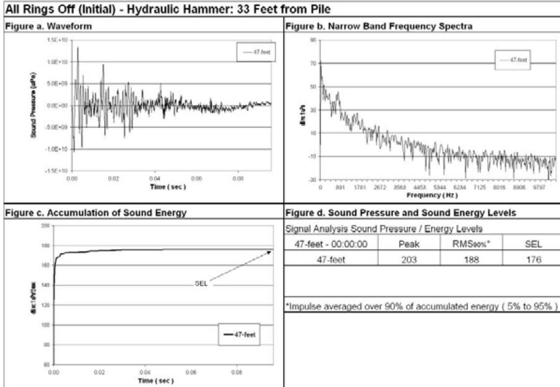
**Figure 77 Waveform Analysis for Pile Number 3, 47-foot Deep (bottom), 33-Feet from Pile, All Rings Off.**
