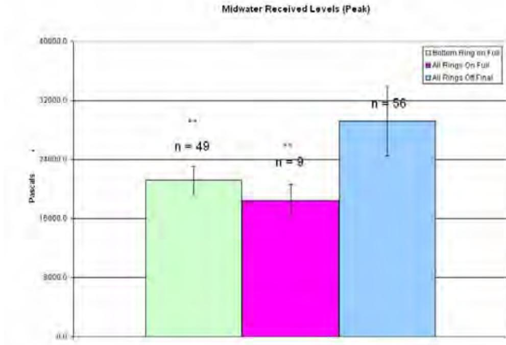
**Figure 39. Pile 8, midwater average peak received levels. Error bars represent one standard deviation. \* = Significant compared to bubbles off initial ( $p < 0.05$ ). \*\* Significant compared to bubbles off final ( $p < 0.05$ )**
