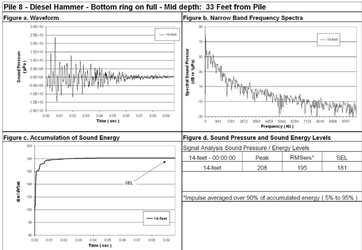
**Figure 106: Waveform Analysis for Pile Number 8, 14-Foot Deep, 33-Foot from Pile, Bottom Ring on full.**
