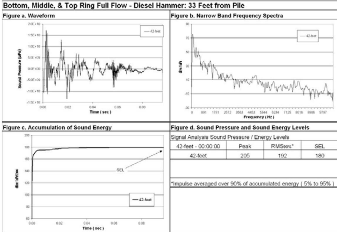
**Figure 67 Waveform Analysis for Pile Number 1, 42-foot Deep (bottom), 33-Foot from Pile, All Rings Off (Final).**
