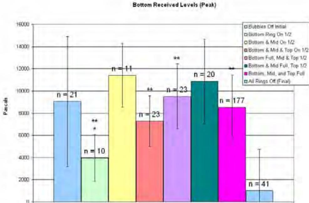
**Figure 8: Pile 1, bottom average peak received levels. Error bars represent one standard deviation. \* = Significant compared to bubbles off initial ( $p < 0.05$ ). \*\* Significant compared to bubbles off final ( $p < 0.05$ ).**
