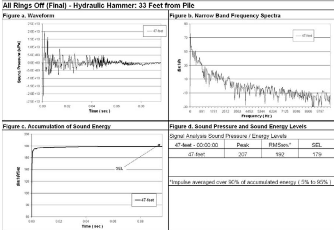
**Figure 83 Waveform Analysis for Pile Number 3, 47-foot Deep (Bottom), 33-Feet from Pile, All Rings Off (Final).**
