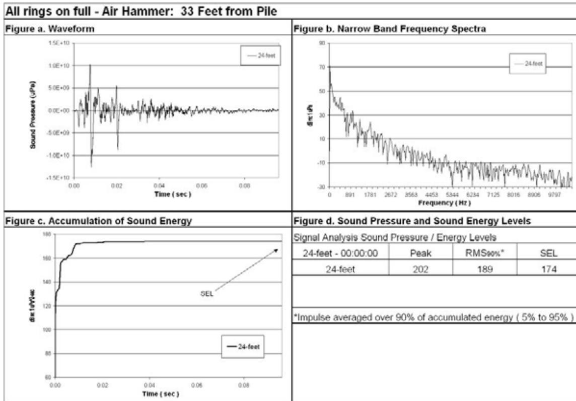
**Figure 70 Waveform Analysis for Pile Number 2, 24-Foot Deep, 33-Foot from Pile, Bottom Ring On Full.**
