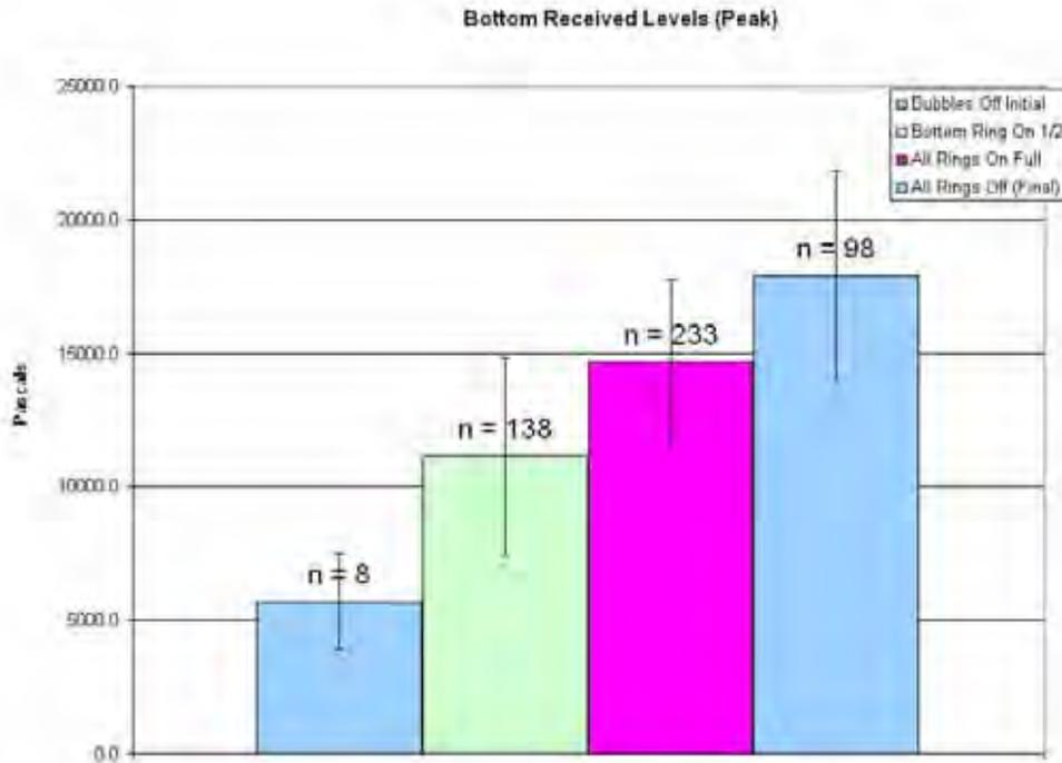
**Figure 14: Pile 2, bottom average peak received levels. Error bars represent one standard deviation. \* = Significant compared to bubbles off initial ( $p < 0.05$ ). \*\* Significant compared to bubbles off final ( $p < 0.05$ )**
