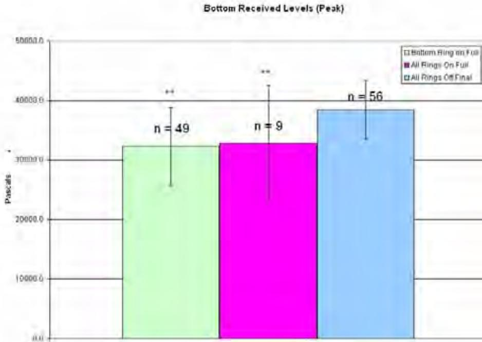
**Figure 40. Pile 1, bottom average peak received levels. Error bars represent one standard deviation. \* = Significant compared to bubbles off initial ( $p < 0.05$ ). \*\* Significant compared to bubbles off final ( $p < 0.05$ )**
