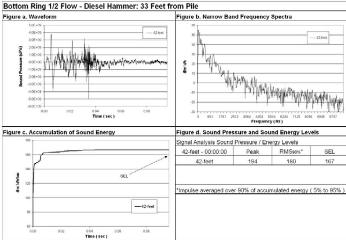
**Figure 55: Waveform Analysis for Pile Number 1, 42-foot Deep (Bottom), 33-Foot from Pile, Bottom Ring 1/2 Flow.**
