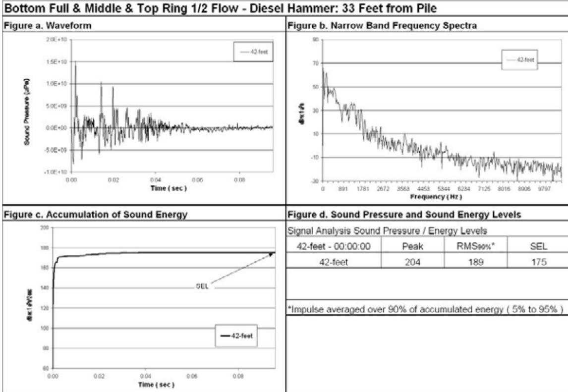
**Figure 61 Waveform Analysis for Pile Number 1, 42-foot Deep (bottom), 33-Feet from Pile, Bottom Ring Full, Middle, and Top Ring 1/2 Flow.**
