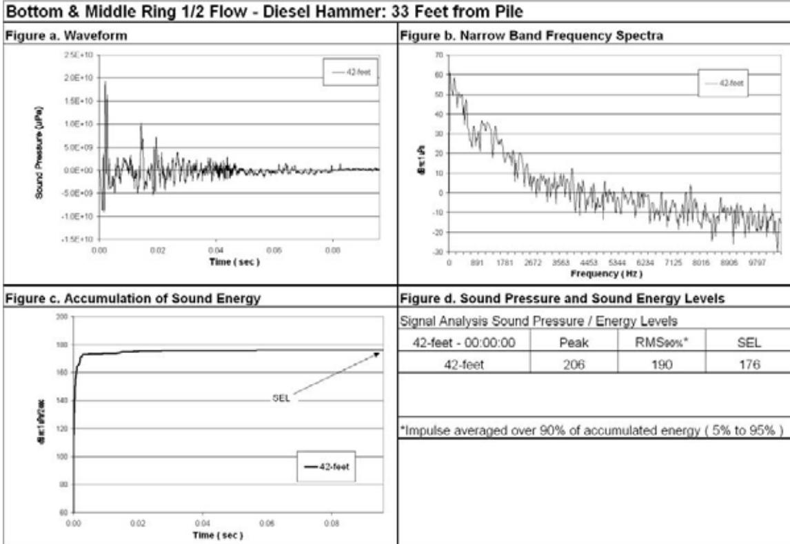
**Figure 57: Waveform Analysis for Pile Number 1, 42-foot Deep (Bottom), 33-Foot from Pile, Bottom and Middle Ring 1/2 Flow.**
