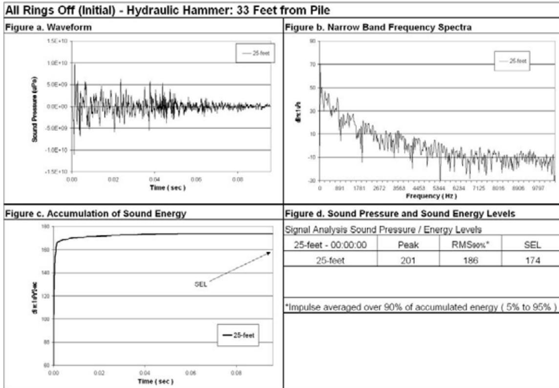
**Figure 76 Waveform Analysis for Pile Number 3, 25-foot Deep, 33-Foot from Pile, All Rings Off (Initial).**
