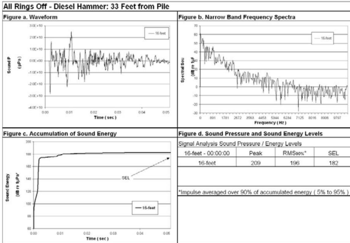
Figure 88: Waveform Analysis for Pile Number 4, 16-Foot Deep, 33-Foot from Pile, All Rings Off.
