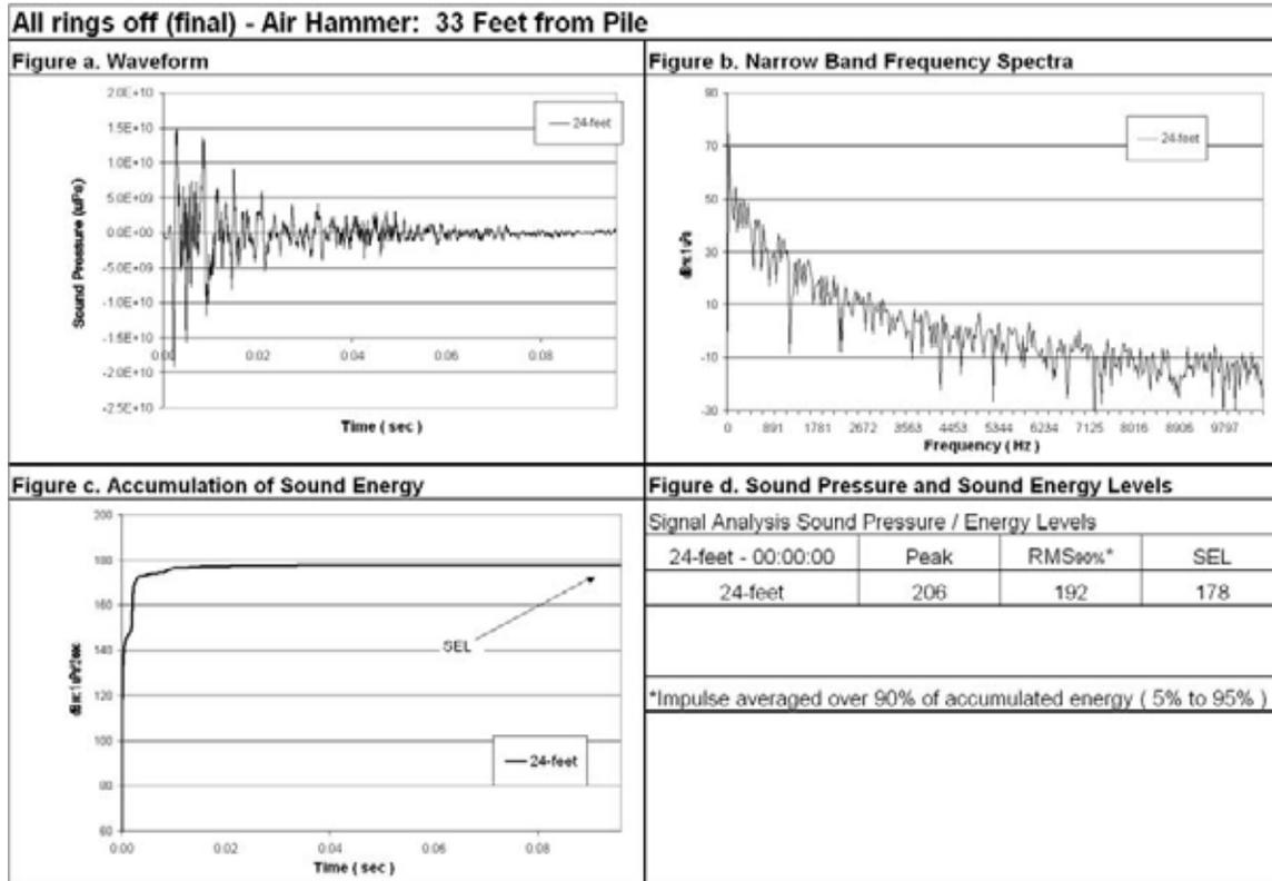
Figure 74 Waveform Analysis for Pile Number 2, 24-Foot Deep, 33-Foot from Pile, All Rings Off (Final).
