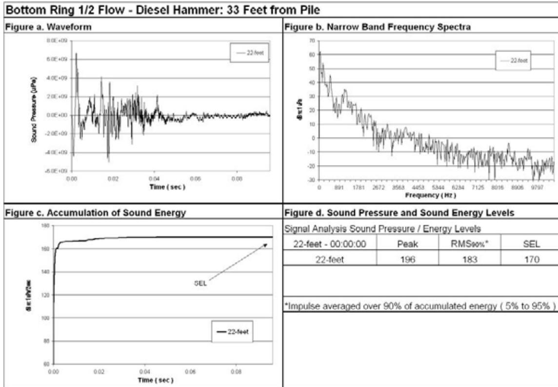
**Figure 54: Waveform Analysis for Pile Number 1, 22-Foot Deep, 33-Foot from Pile, Bottom Ring 1/2 Flow.**
