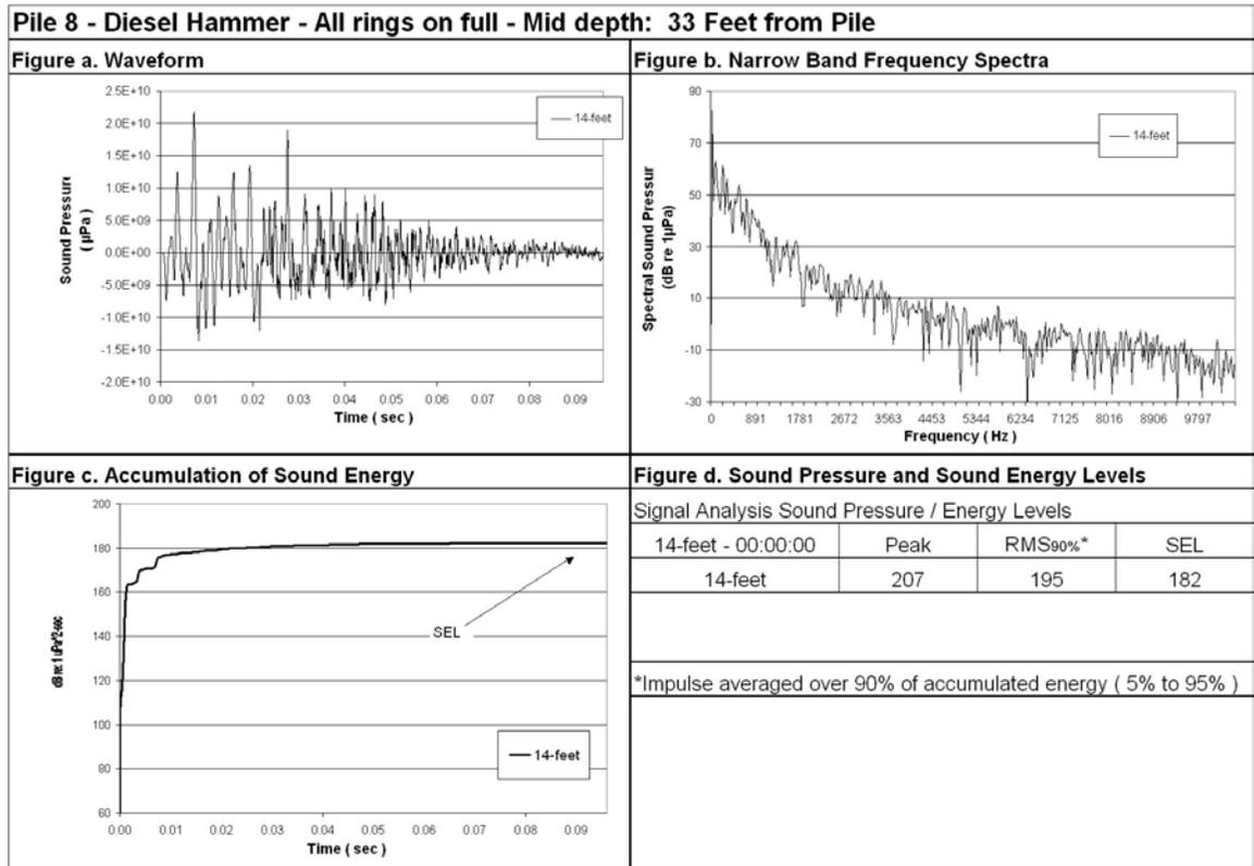
**Figure 108: Waveform Analysis for Pile Number 8, 14-Foot Deep, 33-Foot from Pile, All Rings On Full.**
