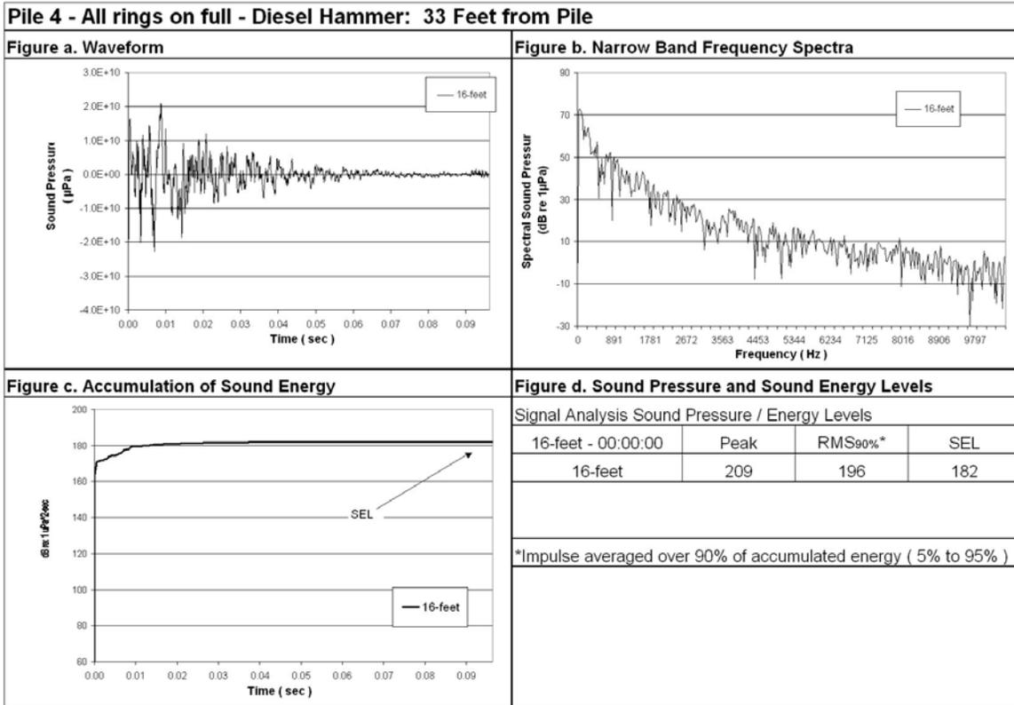
**Figure 86: Waveform Analysis for Pile Number 4, 16-Foot Deep, 33-Foot from Pile, All Rings On Full.**
