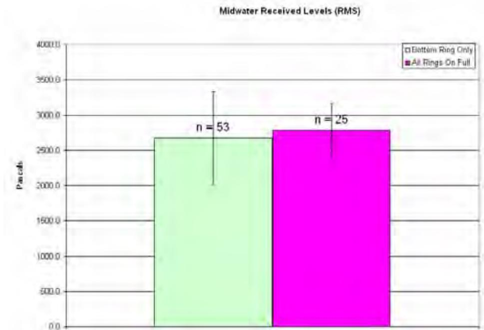
**Figure 37. Pile 7, midwater average RMS received levels. Error bars represent one standard deviation. \* = Significant compared to bottom ring on only ( $p < 0.05$ ).**
