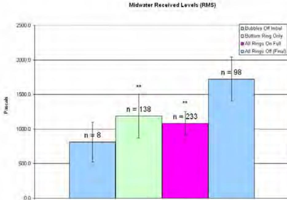
Figure 15: Pile 2, midwater average RMS received levels. Error bars represent one standard deviation. \* = Significant compared to bubbles off initial ( $p < 0.05$ ). \*\* Significant compared to bubbles off final ( $p < 0.05$ )
