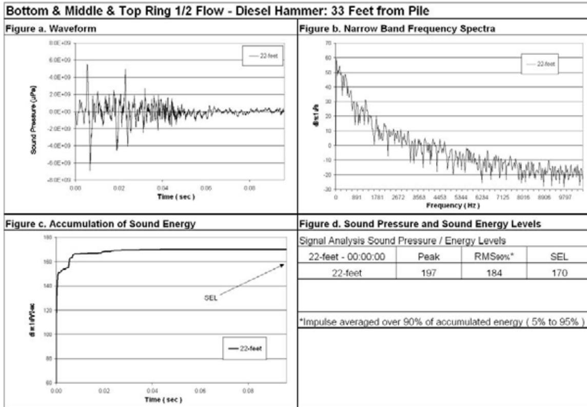
**Figure 58 Waveform Analysis for Pile Number 1, 22-foot Deep, 33-Foot from Pile, Bottom, Middle, and Top Ring 1/2 Flow.**
