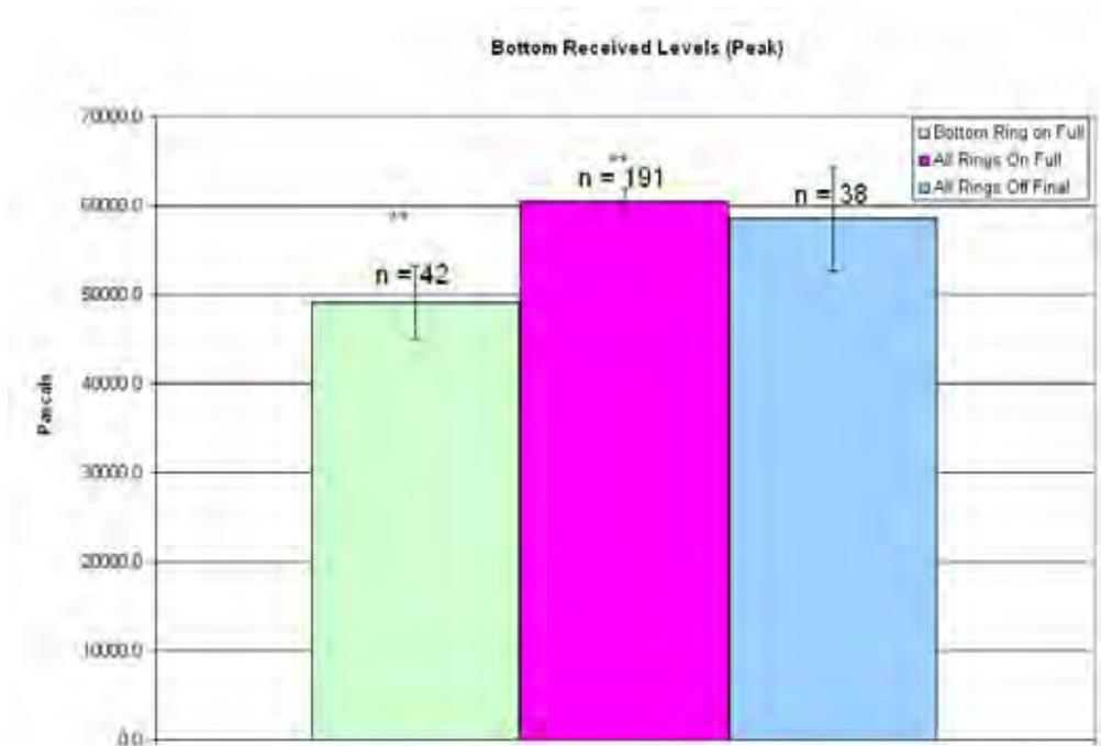
**Figure 27. Pile 5, midwater average peak received levels. Error bars represent one standard deviation. \* = Significant compared to bubbles off initial ( $p < 0.05$ ). \*\* Significant compared to bubbles off final ( $p < 0.05$ )**
