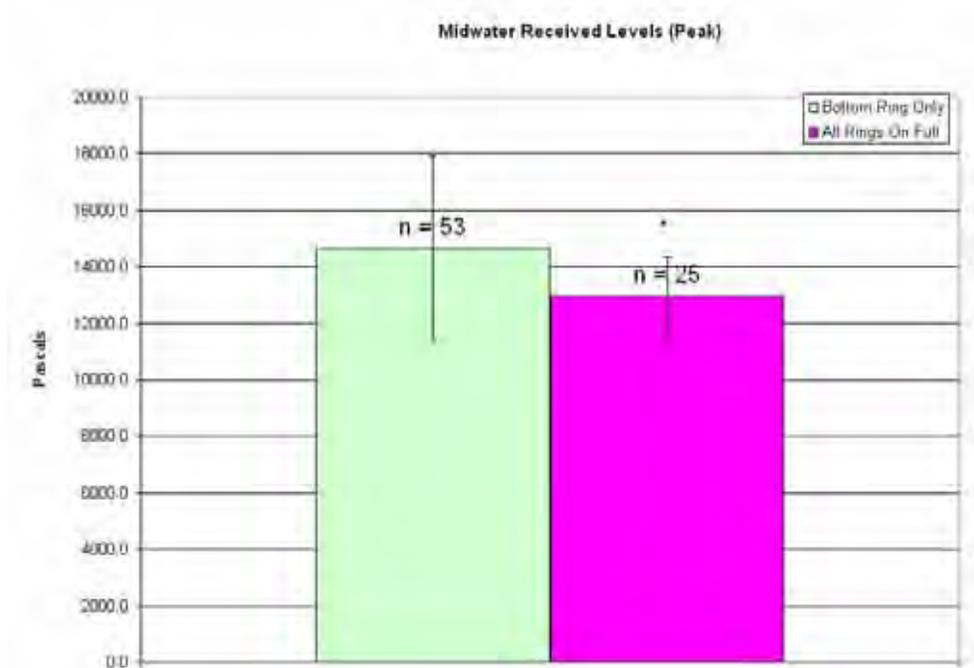
**Figure 35. Pile 7, midwater average peak received levels. Error bars represent one standard deviation. \* = Significant compared to bbottom ring on only (p<0.05).**
