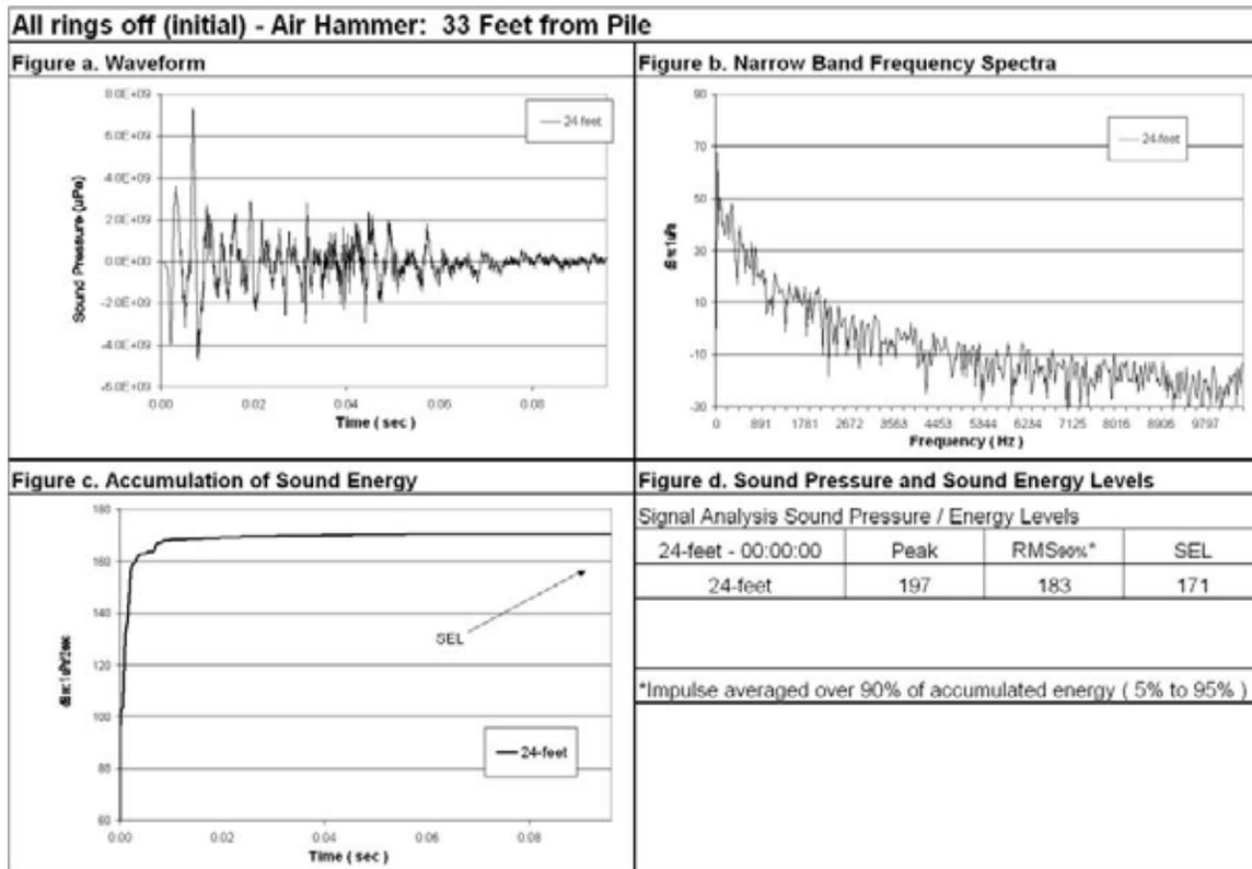
**Figure 68: Waveform Analysis for Pile Number 2, 24-Foot Deep, 33-Foot from Pile, All Rings Off.**
