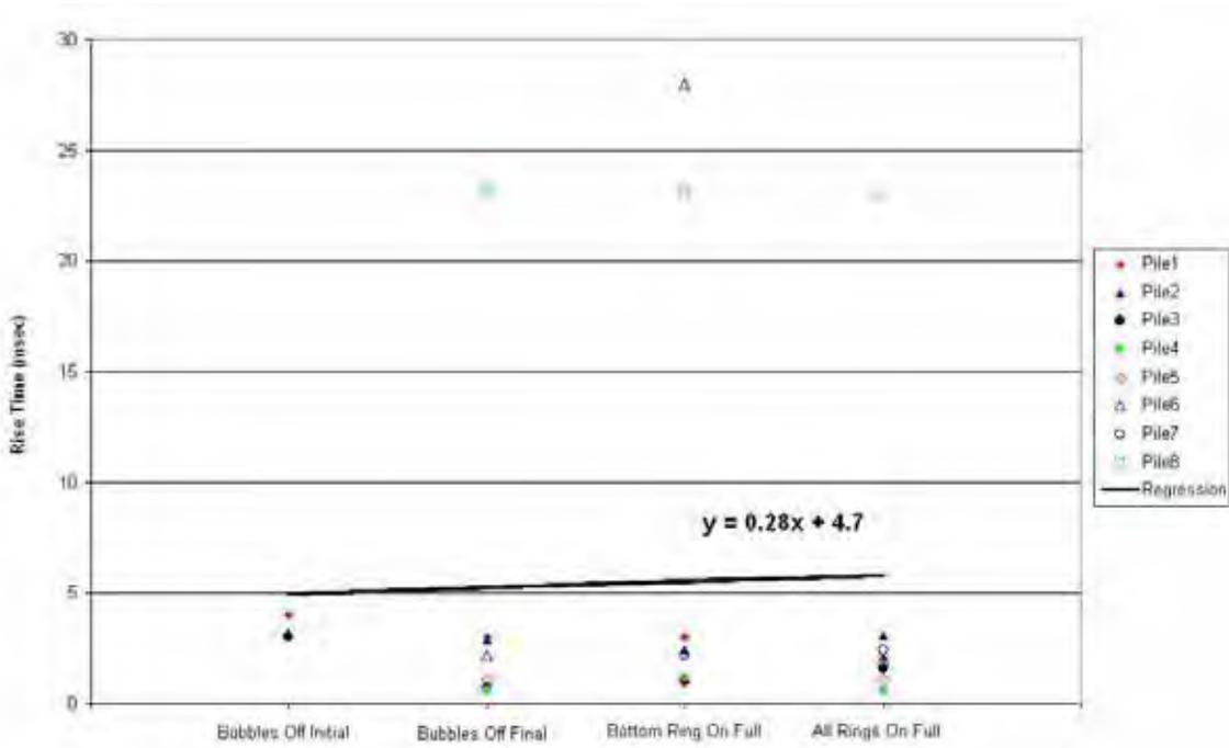
**Figure 45. Rise times for each bottom received level peak pile strike with linear regression line.**
