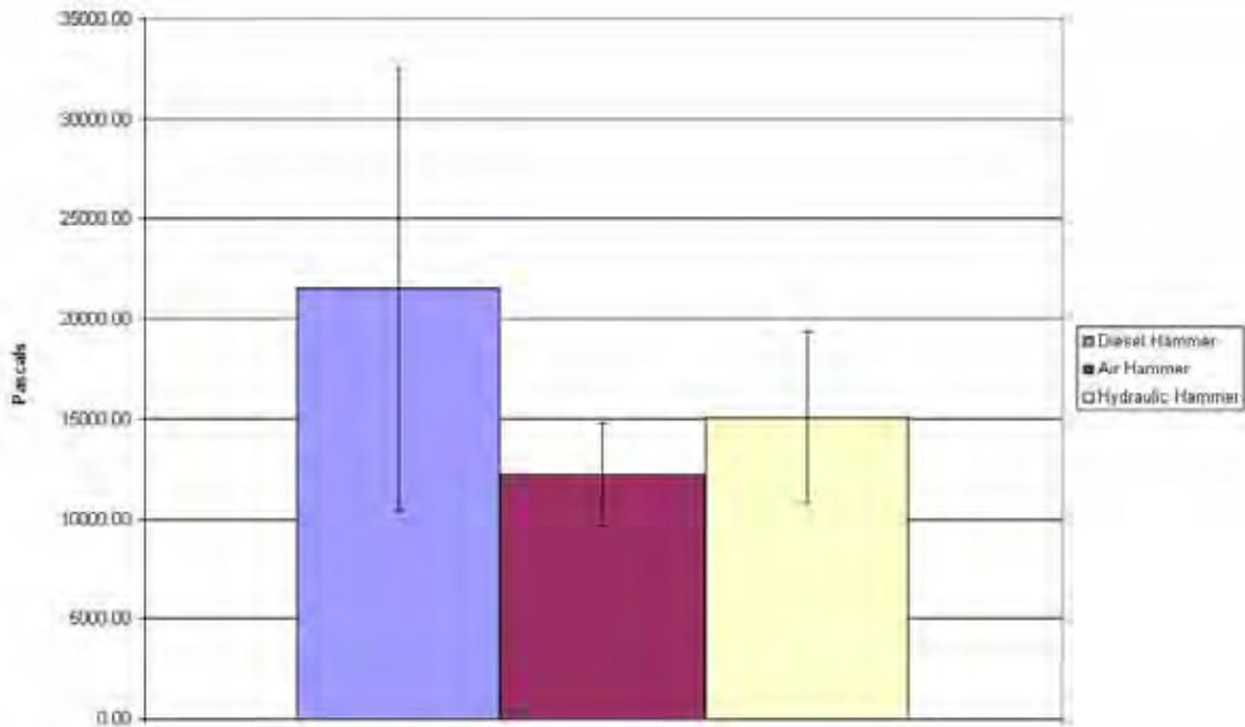
**Figure 46. Average absolute peak midwater received values for each hammer type, all bubble rings off. Error bars are  $\pm$  one standard deviation.**
