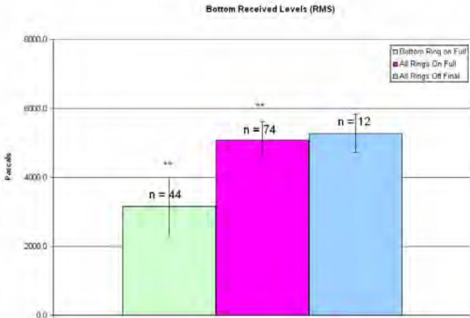
**Figure 25: Pile 4, bottom average RMS received levels. Error bars represent one standard deviation. \* = Significant compared to bubbles off initial ( $p < 0.05$ ). \*\* Significant compared to bubbles off final ( $p < 0.05$ )**
