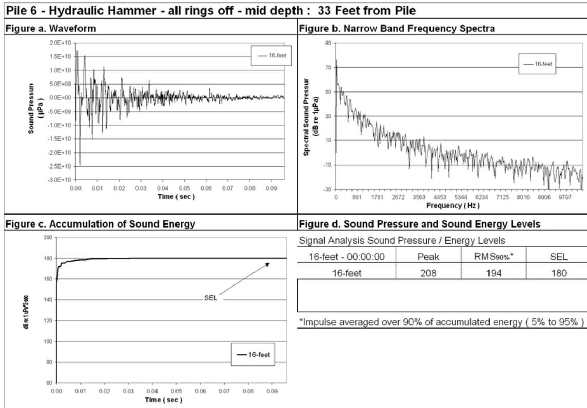
**Figure 100: Waveform Analysis for Pile Number 6, 16-Foot Deep, 33-Foot from Pile, All Rings Off.**
