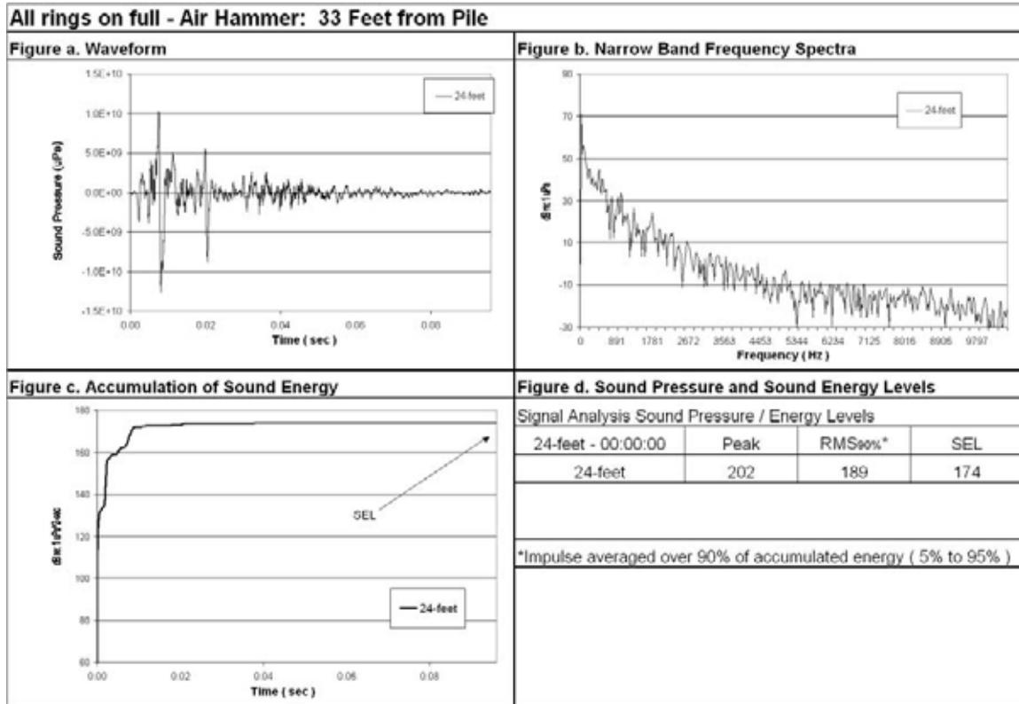
**Figure 72 Waveform Analysis for Pile Number 2, 24-Foot Deep, 33-Foot from Pile, All Rings On Full.**
