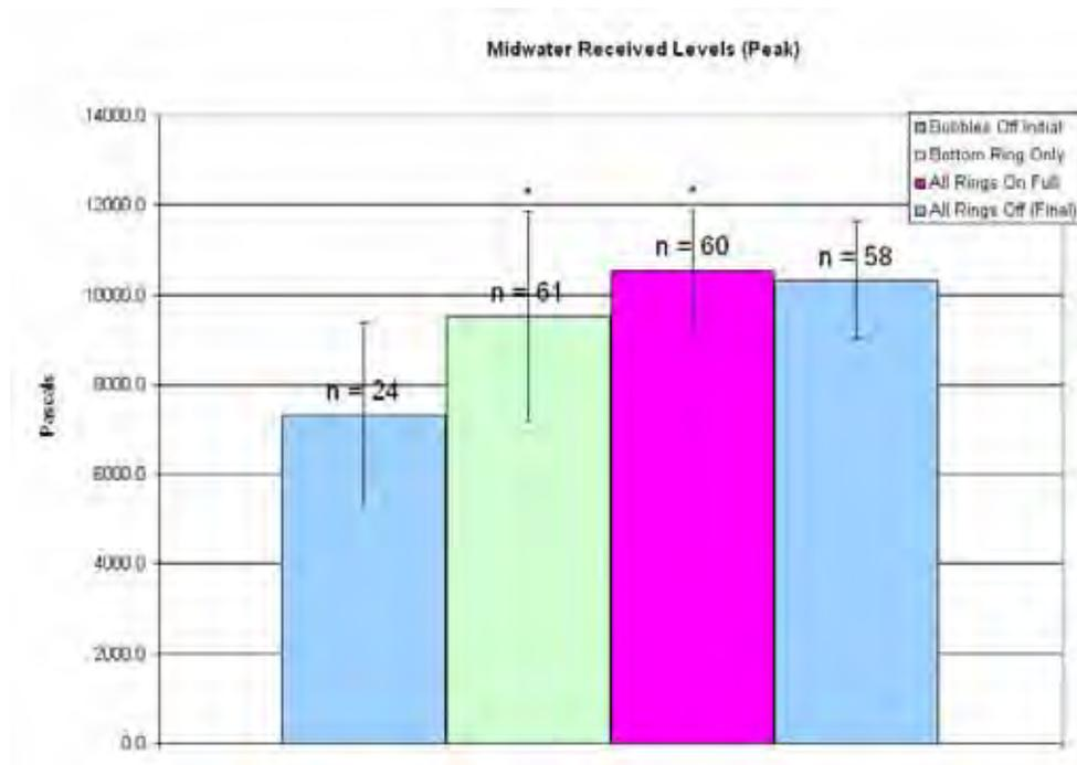
**Figure 17: Pile 3, midwater average peak received levels. Error bars represent one standard deviation. \* = Significant compared to bubbles off initial ( $p < 0.05$ ). \*\* Significant compared to bubbles off final ( $p < 0.05$ )**
