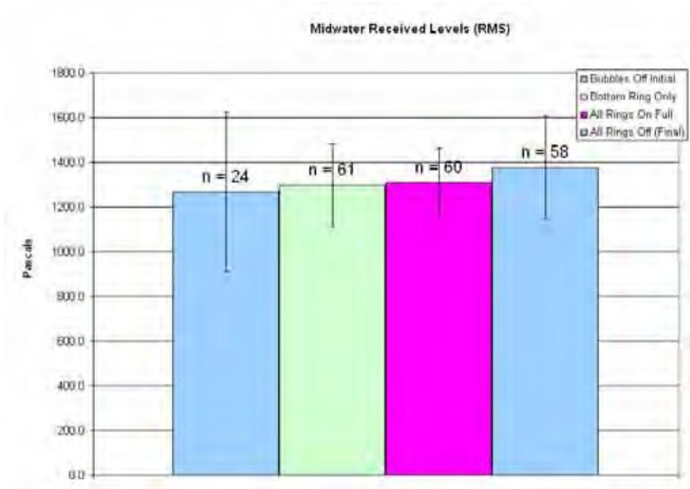
**Figure 19: Pile 3, midwater average RMS received levels. Error bars represent one standard deviation. \* = Significant compared to bubbles off initial ( $p < 0.05$ ). \*\* Significant compared to bubbles off final ( $p < 0.05$ )**
