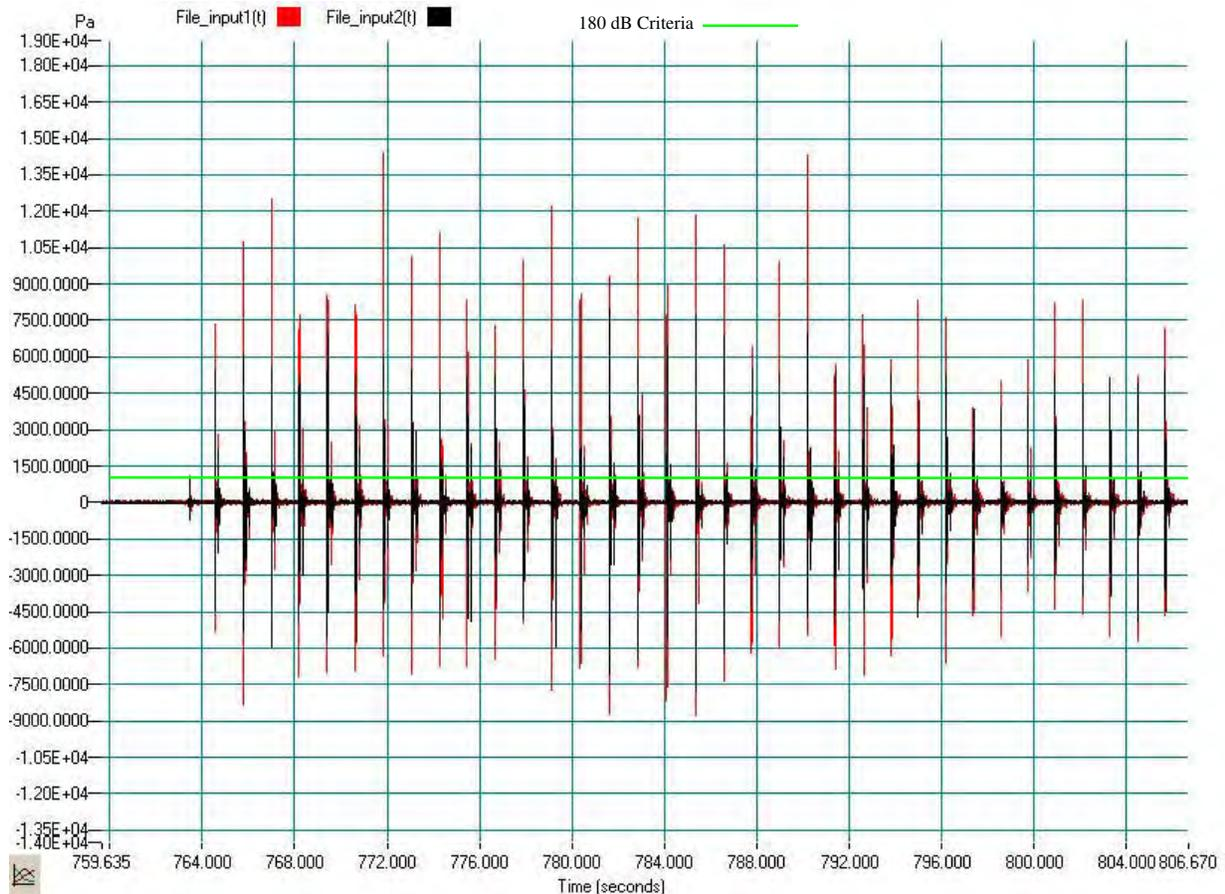
**Figure 6: Pile 1 Initial Pile Strikes with Bubble Curtain On Full. (File\_input1(t) = bottom; File\_input2(t) = midwater)**
