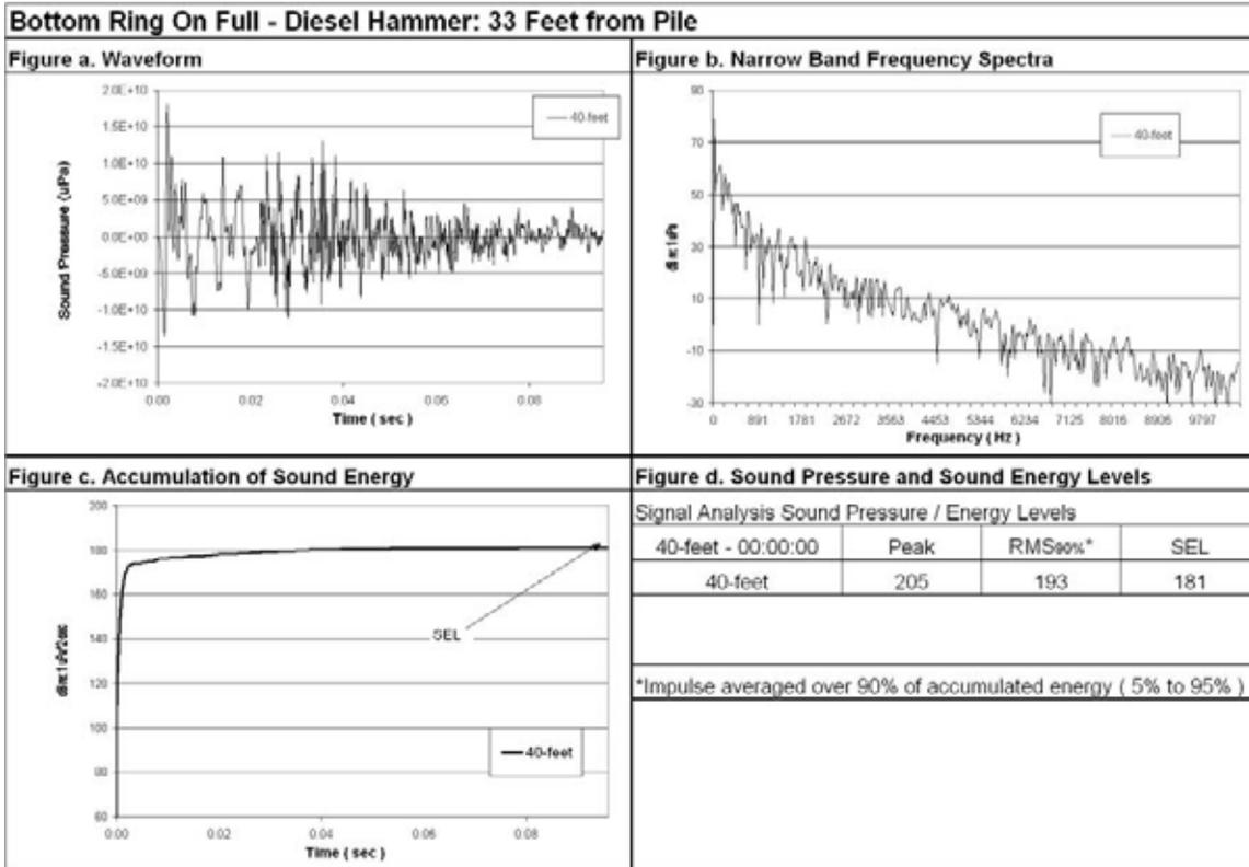
**Figure 103: Waveform Analysis for Pile Number 7, 40-Foot Deep (Bottom), 33-Foot from Pile, Bottom Ring On Full.**
