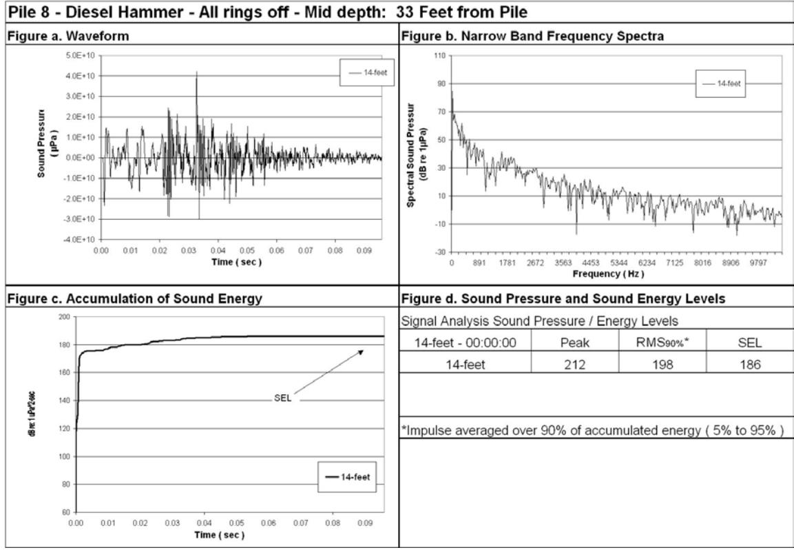
**Figure 110: Waveform Analysis for Pile Number 8, 14-Foot Deep, 33-Foot from Pile, All Rings Off.**
