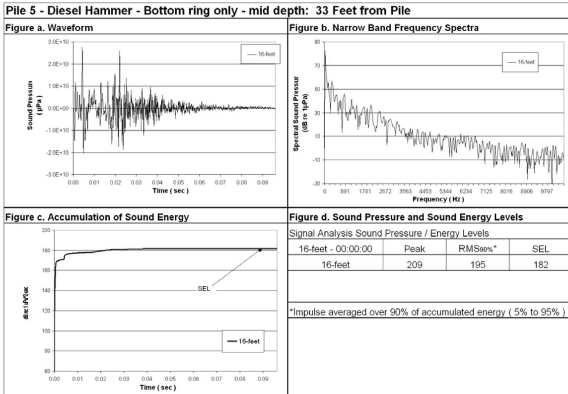
**Figure 90: Waveform Analysis for Pile Number 5, 16-feet Deep, 33-Foot from Pile, Bottom Ring On Full.**
