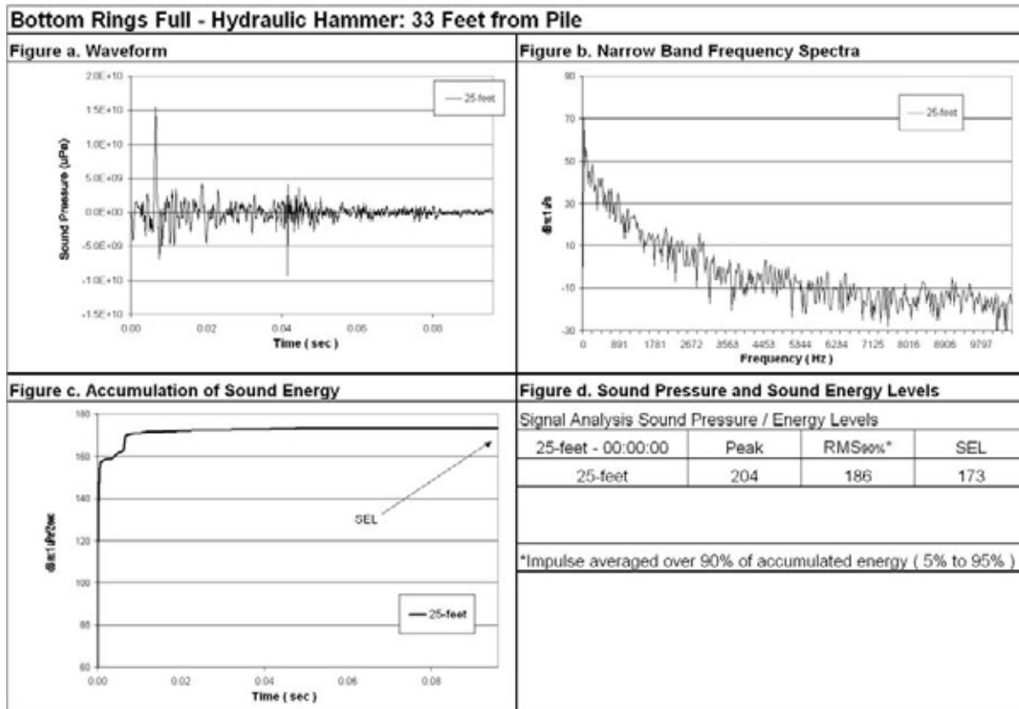
**Figure 78 Waveform Analysis for Pile Number 3, 25-feet Deep, 33-Foot from Pile, Bottom Ring On Full.**
