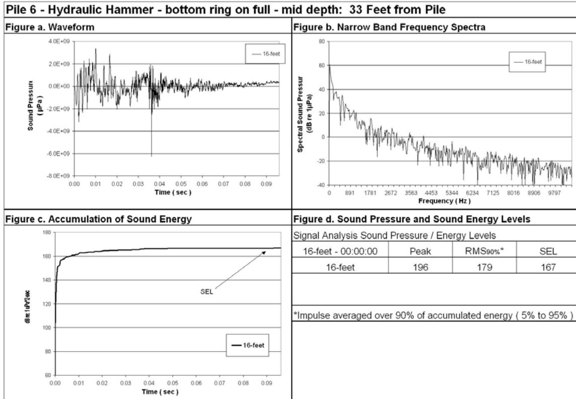
**Figure 96: Waveform Analysis for Pile Number 6, 16-Foot Deep, 33-Foot from Pile, Bottom Ring On Full.**
