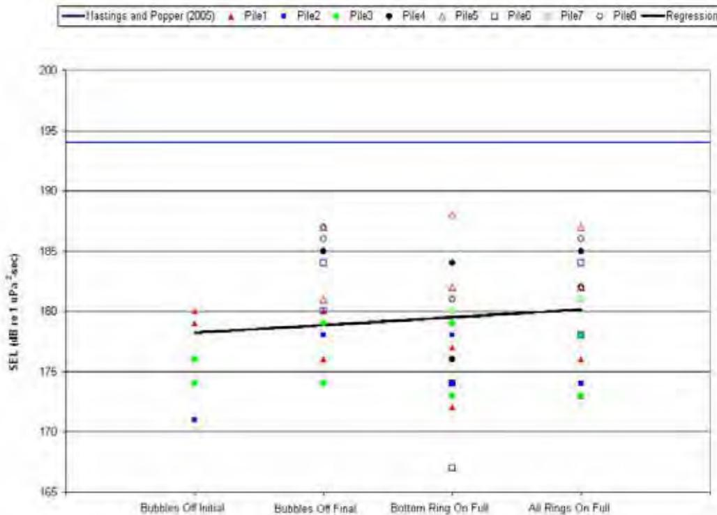
**Figure 43. SEL values for each pile compared with the 194 dB SEL proposed threshold from Hastings and Popper (2005). Regression line formula is:  $y=0.639X + 177.6$ .**
