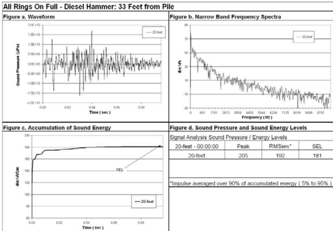
Figure 104: Waveform Analysis for Pile Number 7, 20-Foot Deep, 33-Foot from Pile, All Rings On Full.
