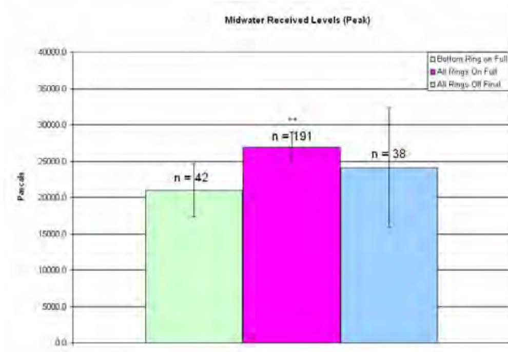
**Figure 26. Pile 5, midwater average peak received levels. Error bars represent one standard deviation. \* = Significant compared to bubbles off initial ( $p < 0.05$ ). \*\* Significant compared to bubbles off final ( $p < 0.05$ )**
