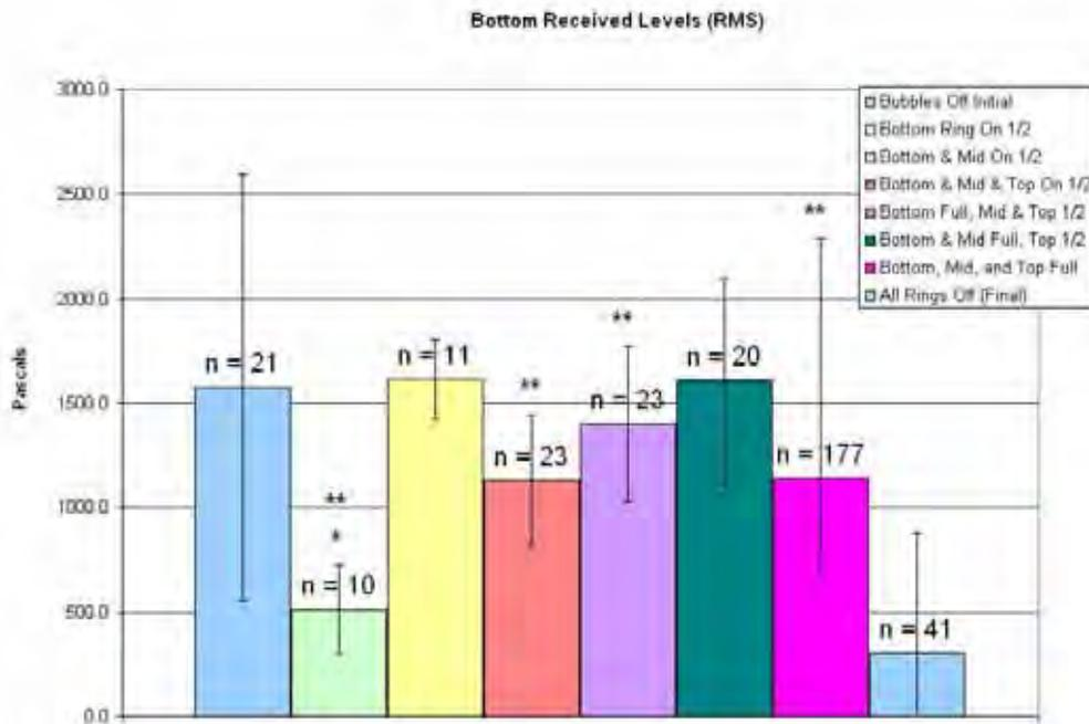
Figure 10: Pile 1, bottom average RMS received levels. Error bars represent one standard deviation. \* = Significant compared to bubbles off initial ( $p < 0.05$ ). \*\* Significant compared to bubbles off final ( $p < 0.05$ ).
