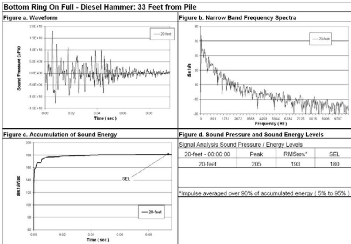
**Figure 102: Waveform Analysis for Pile Number 7, 20-Foot Deep, 33-Foot from Pile, Bottom Ring On Full.**
