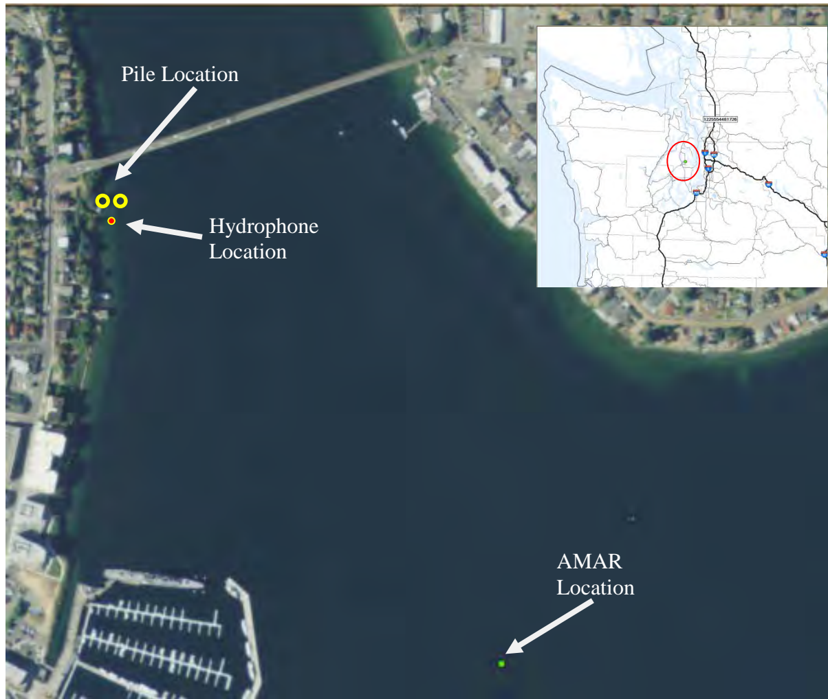
Figure 1: Approximate locations of near field and far field (AMAR) monitoring locations at the Manette Bridge. ● = Approximate pile location
