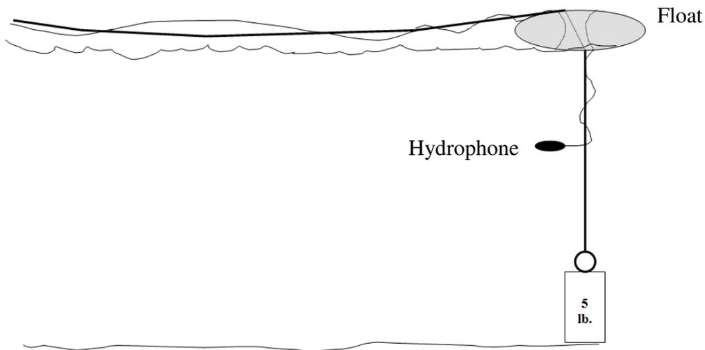
**Figure 4: Diagram of hydrophone deployment configuration.**
