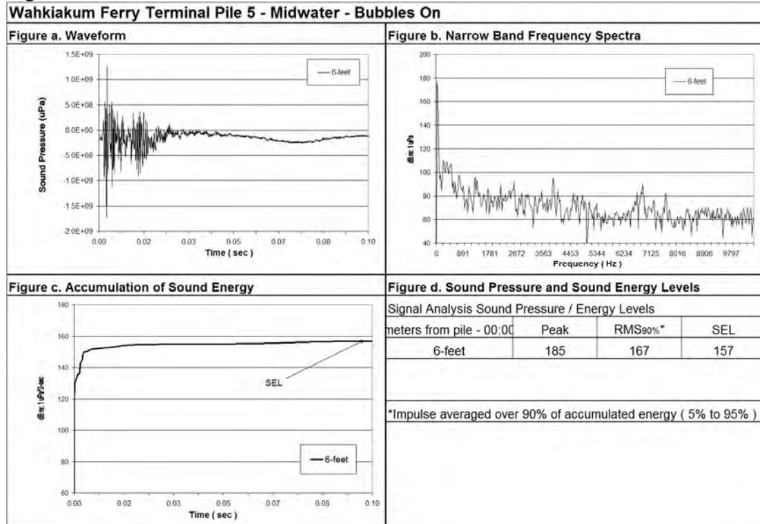
**Figure 15: Waveform analysis of Pile 5 sound pressure levels without (a) and with (b) bubbles, midwater.**
