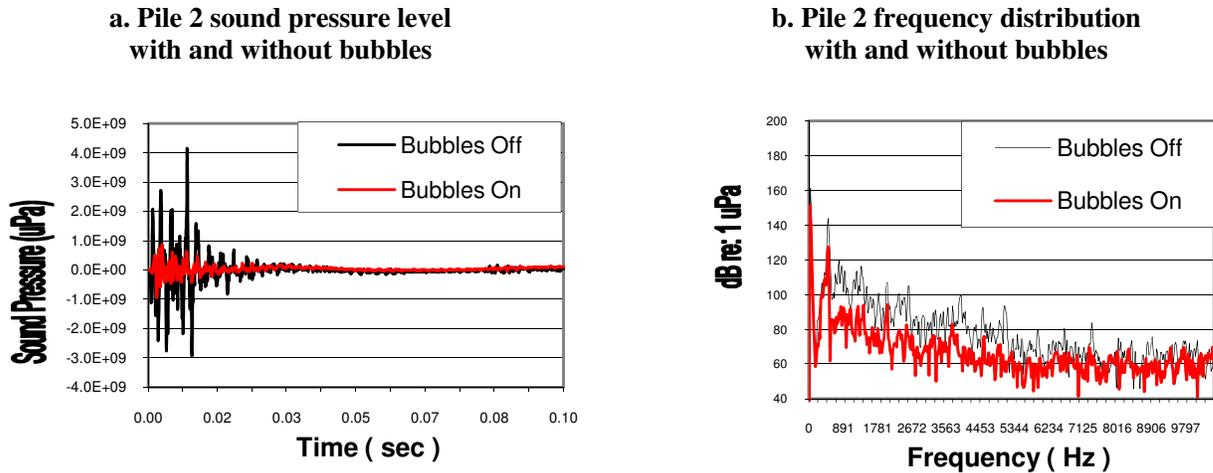
**Figure 6: Waveforms and frequency spectral analysis for pile 2 with bubbles on and off.**
