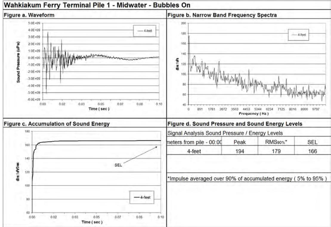
Figure 11: Waveform analysis of Pile 1 sound pressure levels with mitigation, 4 feet water depth.
