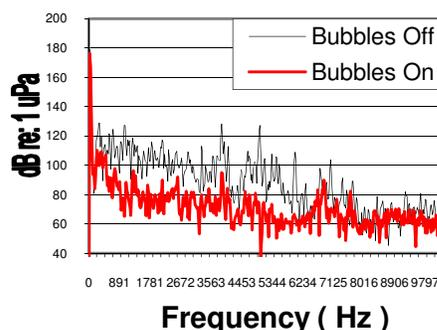
**Figure 9: Waveforms and frequency spectral analysis for pile P-8 using the TNAP.**
