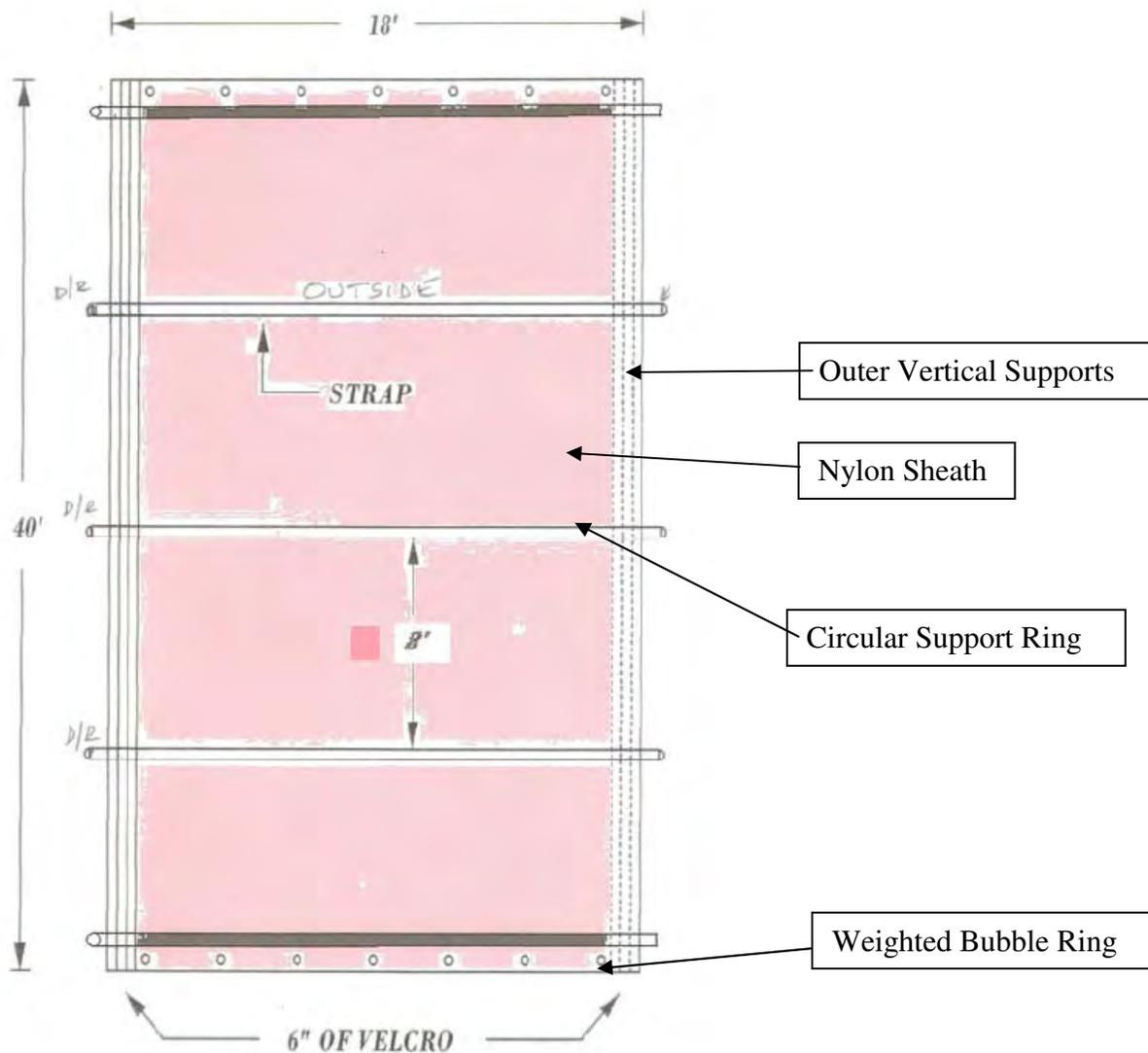
**Figure 5: Diagram of confined bubble curtain.**
