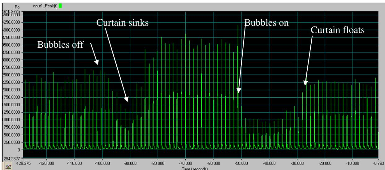
**Figure 10: Chart of peak pile strikes with and without bubbles in confined bubble curtain.**
