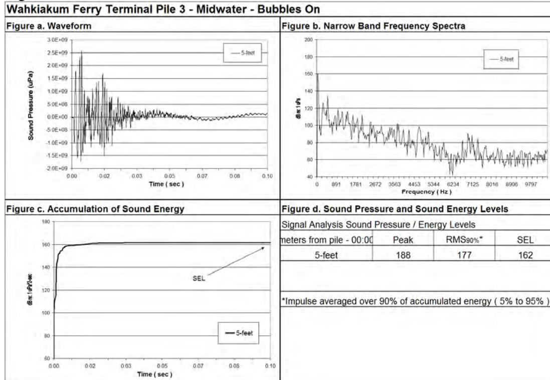
**Figure 13: Waveform analysis of Pile 3 sound pressure levels without (a) and with Bubbles (b), midwater.**
