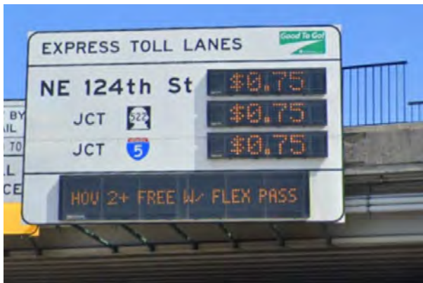
Figure 4. I-405 Variable Message Signs
