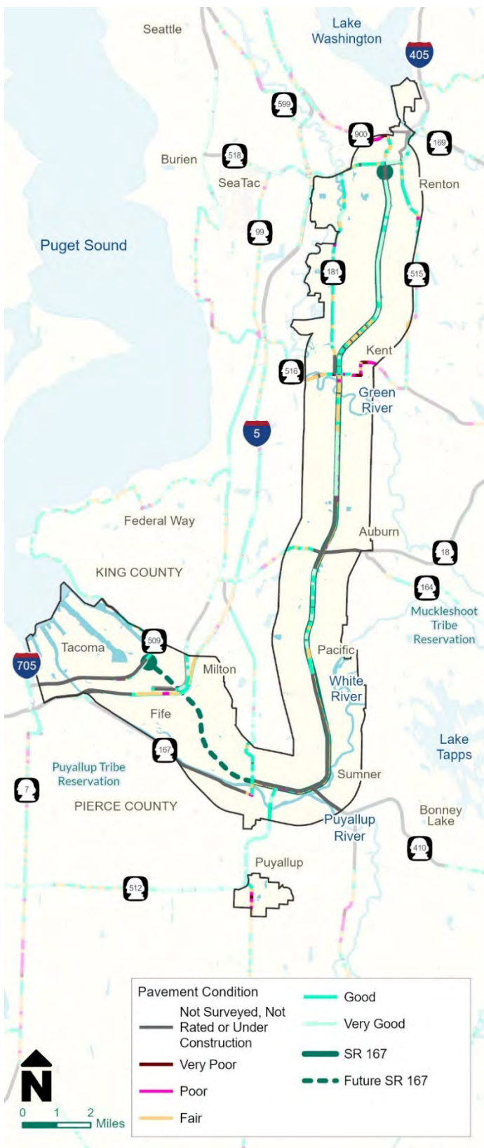
Figure 4-4. SR 167 Pavement Condition
