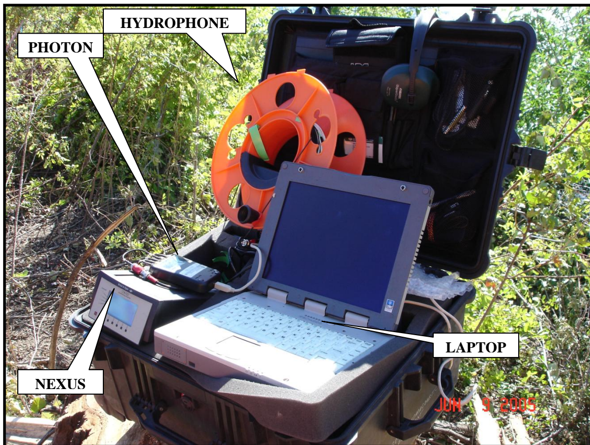
Figure 3: Near field acoustical monitoring equipment
