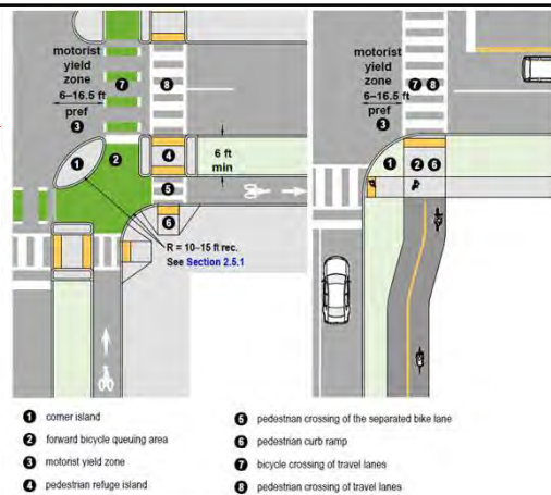
Figure 7-13: Protected Intersection Design for Separated Bike Lanes and Side Paths
