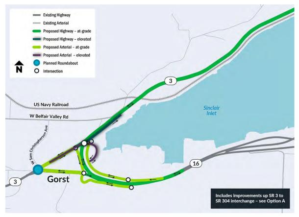
**Alternative A-2** adds an elevated roundabout and two frontage roads through Gorst. Business access is provided by the frontage roads with an overpass between the east and west sides of SR 16. The elevated roundabout and frontage roads would allow regional traffic to continue along the at grade roadway without being disrupted by traffic accessing local businesses and residences.
