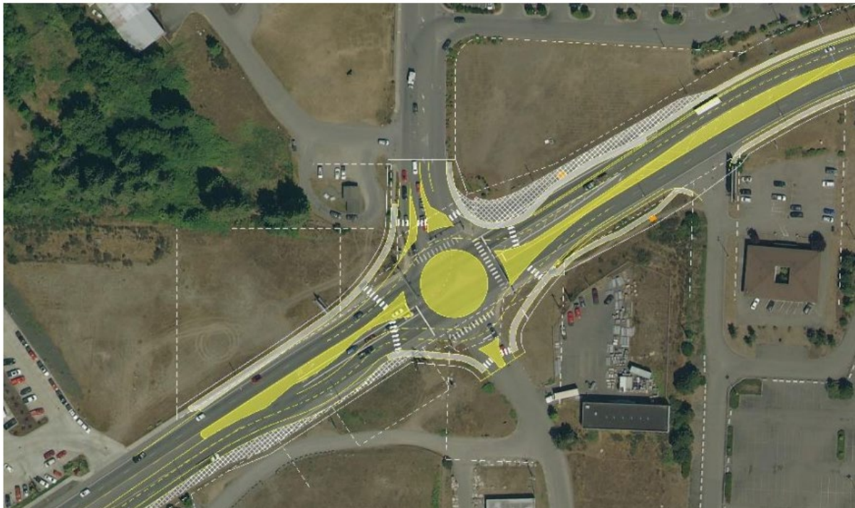
Figure 15: Recommended future two-lane roundabout at East Kolonels Way.
